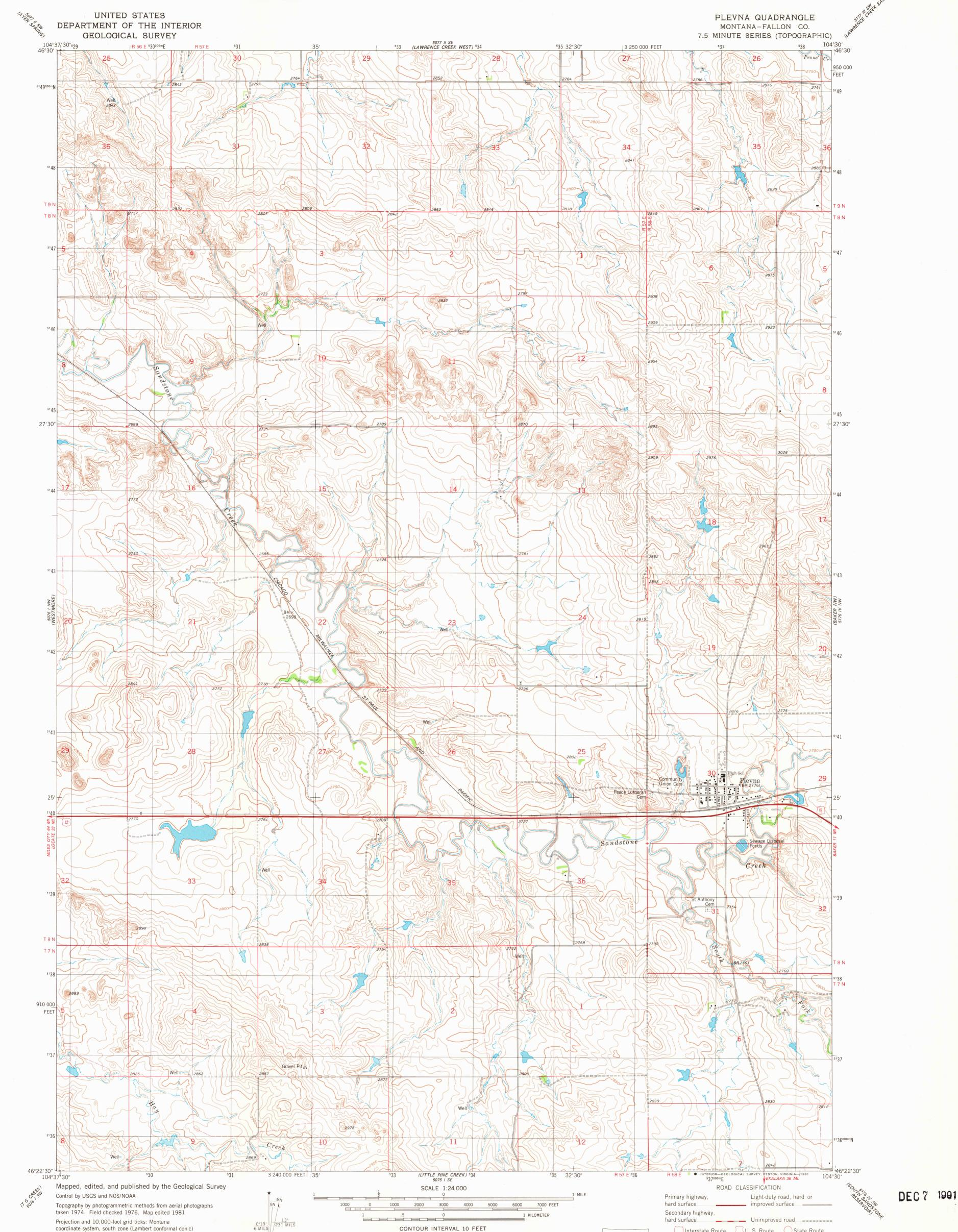
coordinate system, south zone (Lambert conformal conic) 1000-meter Universal Transverse Mercator grid, zone 13 1927 North American datum To place on the predicted North American Datum 1983 move the projection lines 4 meters north and 40 meters east as shown by dashed corner ticks Fine red dashed lines indicate selected fence lines
