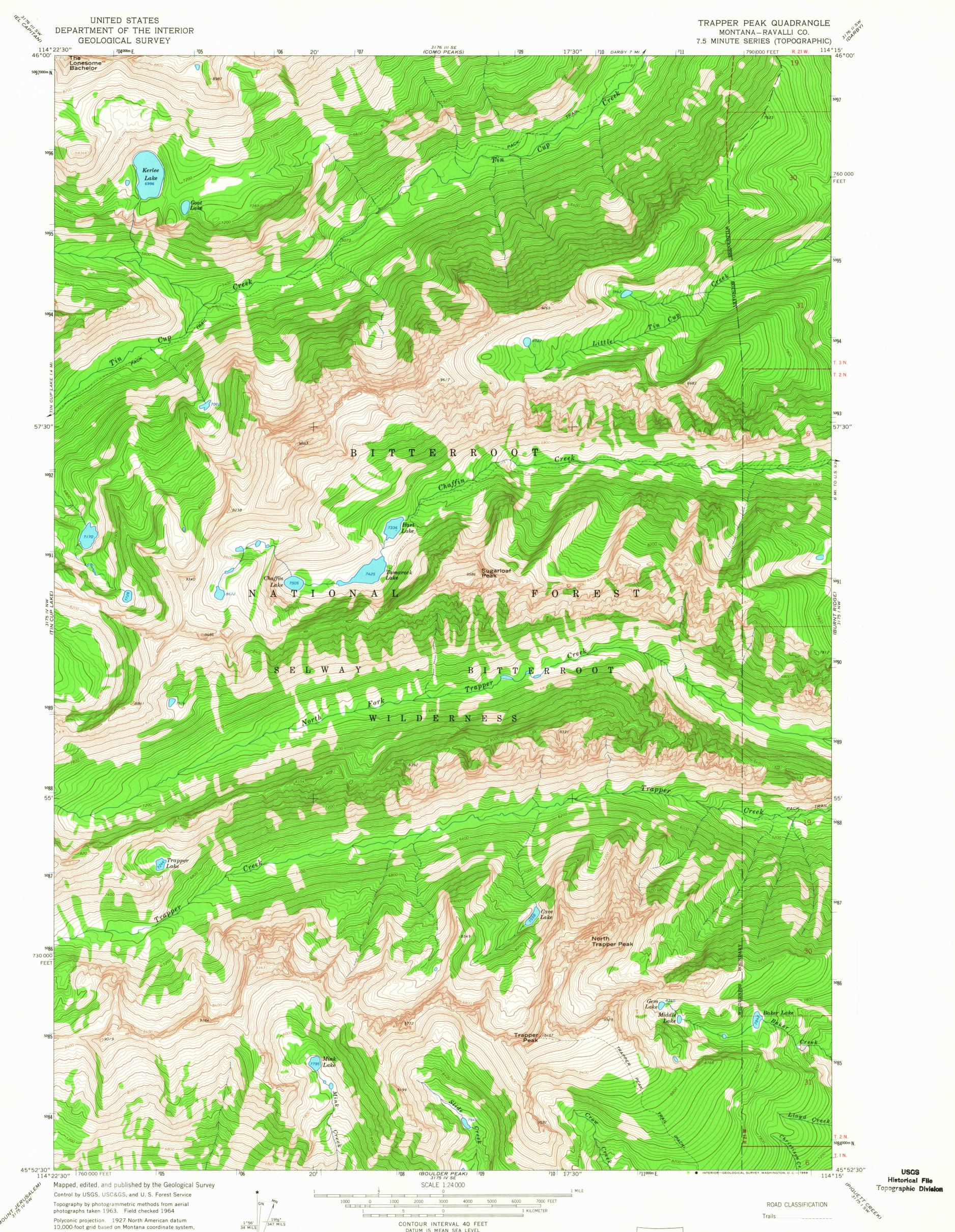
Polyconic projection. 1927 North American datum 10,000-foot grid based on Montana coordinate system, south zone 1000-meter Universal Transverse Mercator grid ticks, zone 11, shown in blue UTM GRID AND 1964 MAGNETIC NORTH DECLINATION AT CENTER OF SHEET Where omitted, land lines have not been established
