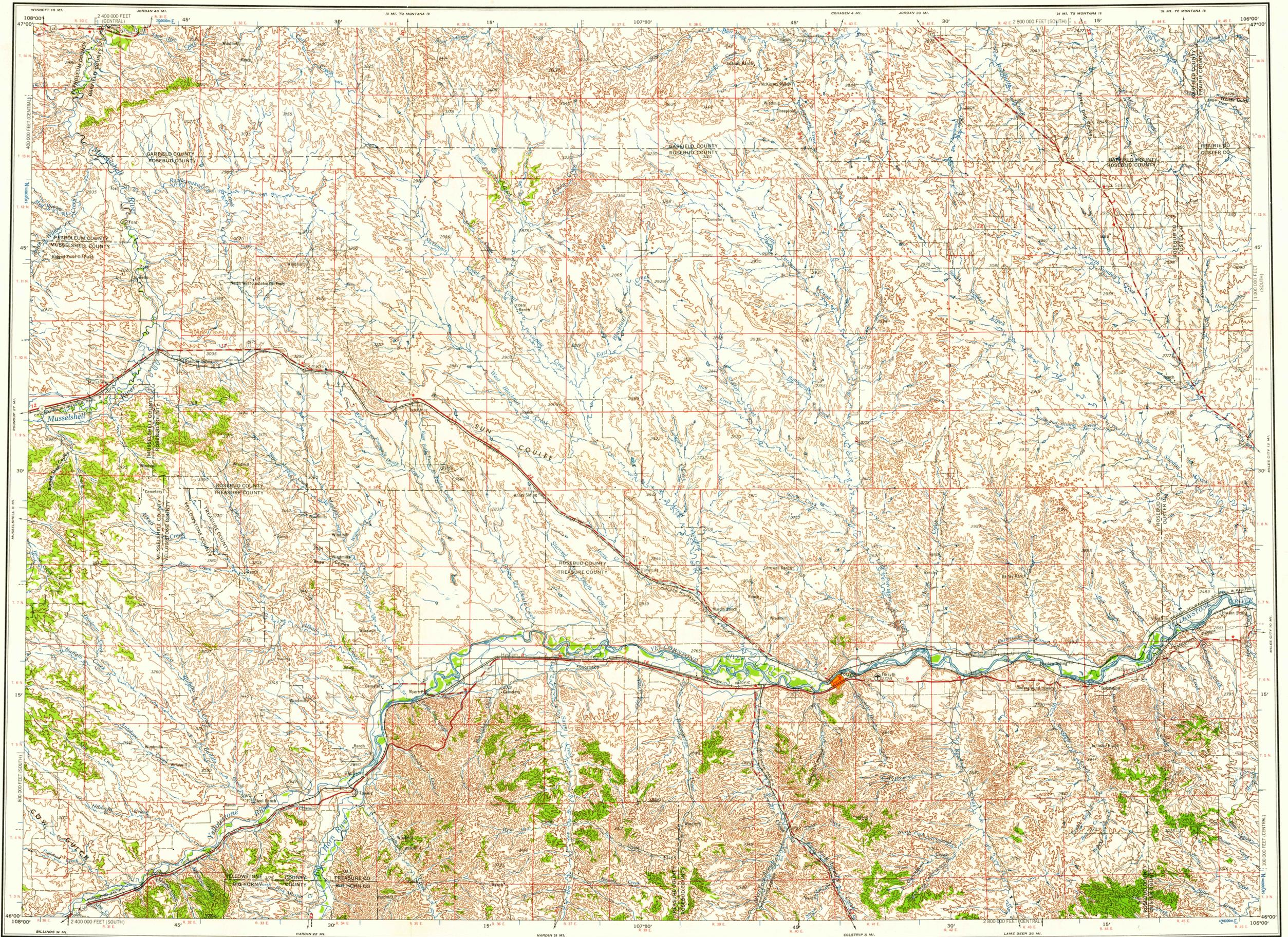
Prepared by the Army Map Service (AJART), Corps of Engineers, U.S. Army, Washington, D.C. Compiled in 1955 by photogrammetric methods. Horizontal and vertical control by USCGS and CE. Aerial photography 1953. Photography field annotated in 1954. 100,000 foot grids based on Montana coordinate system, south and central zones. 10,000 meter Universal Transverse Mercator grid ticks, zone 13, shown in blue.
