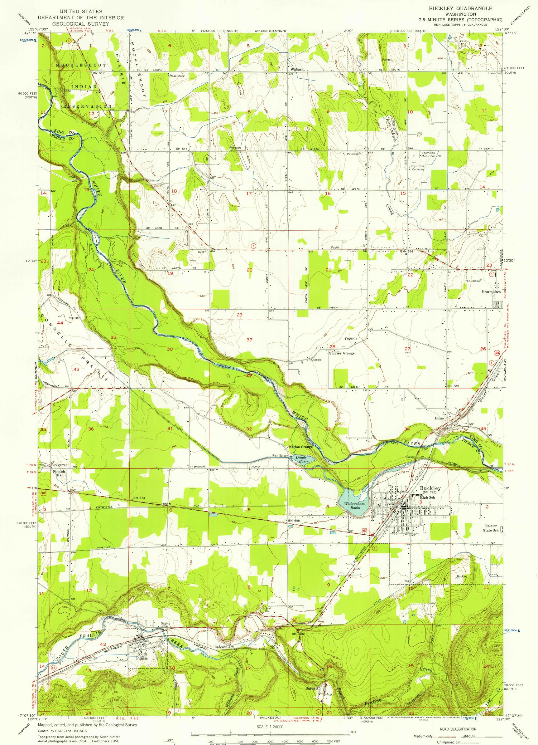
Polyconic projection. 1927 North American datum 10,000-foot grids based on Washington coordinate system, north and south zones 1000-meter Universal Transverse Mercator grid ticks, zone 10, shown in blue
