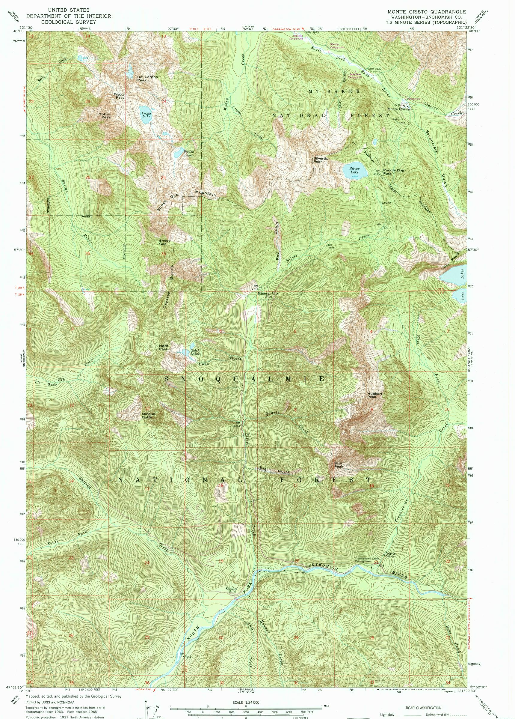
Polyconic projection. 1927 North American datum 10,000-foot grid based on Washington coordinate system, north zone 1000-meter Universal Transverse Mercator grid ticks, zone 10, shown in blue To place on the predicted North American Datum 1983, move the projection lines 22 meters north and 91 meters east as shown by dashed corner ticks Where omitted, land lines have not been established There may be private inholdings within the boundaries of the National or State reservations shown on this map
