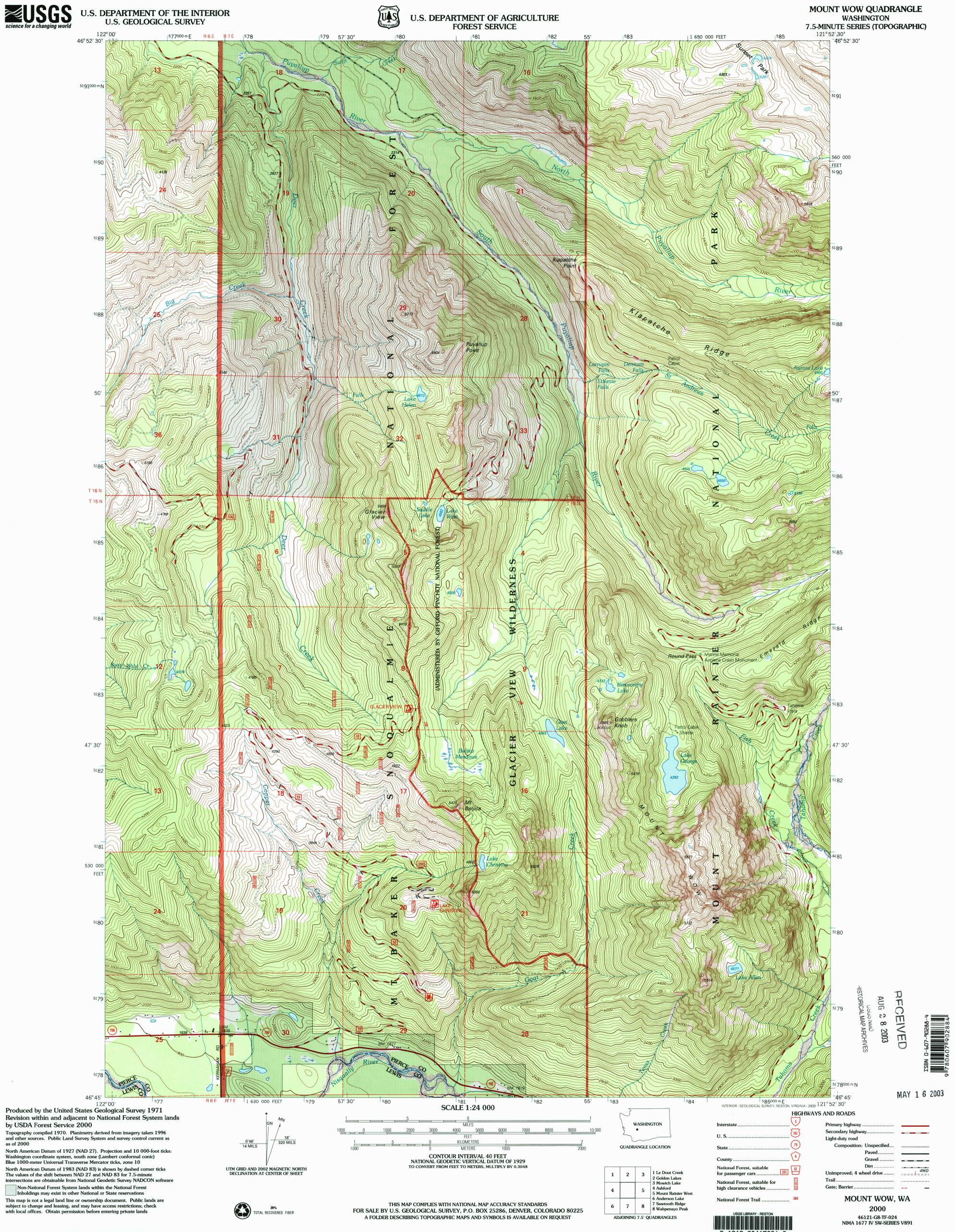
Washington coordinate system, south zone (Lambert conformal conic) Blue 1000-meter Universal Transverse Mercator ticks, zone 10 North American Datum of 1983 (NAD 83) is shown by dashed corner ticks The values of the shift between NAD 27 and NAD 83 for 7.5-minute
