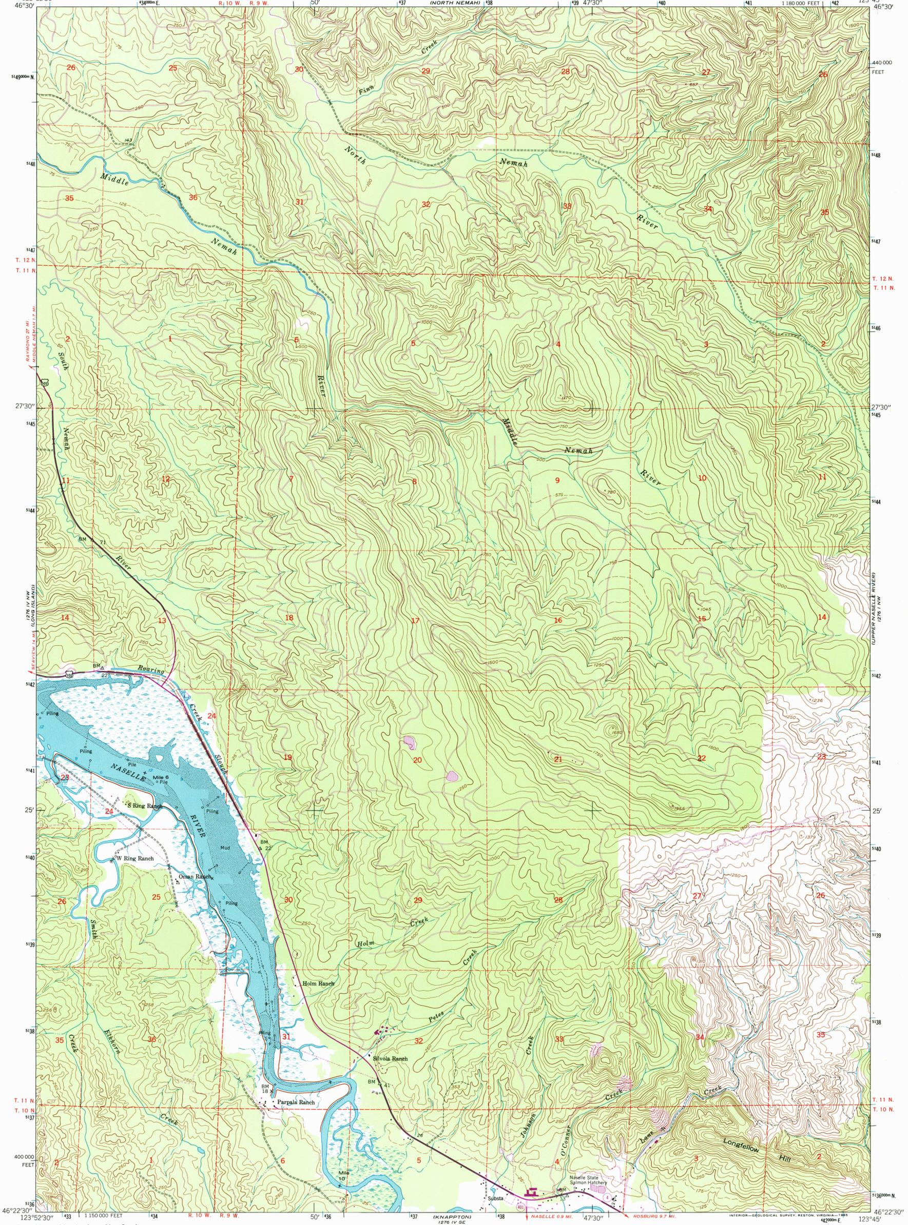
Mapped by the Army Map Service... Topography from aerial photographs by multiplex methods... Aerial photographs taken 1943. Field checked 1949... POLYCONIC PROJECTION. 1927 NORTH AMERICAN DATUM... 10,000-FOOT GRID BASED ON WASHINGTON COORDINATE SYSTEM... UTM GRID AND 1984 MAGNETIC NORTH DECLINATION AT CENTER OF SHEET
