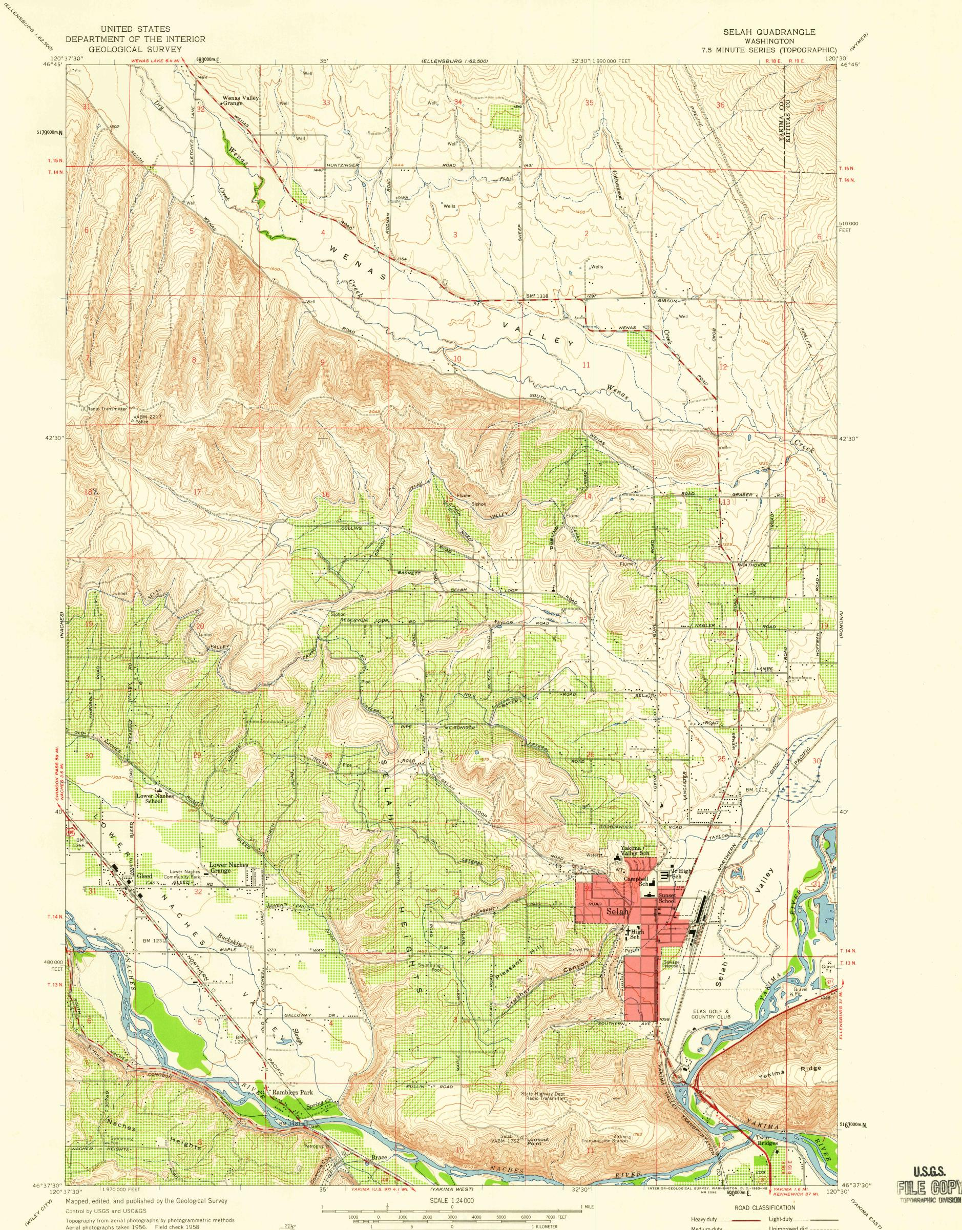
Aerial photographs taken 1956. Field check 1958 Polyconic projection. 1927 North American datum 10,000-foot grid based on Washington coordinate system, south zone 1000-meter Universal Transverse Mercator grid ticks, zone 10, shown in blue Red tint indicates area in which only landmark buildings are shown Unchecked elevations are shown in brown
