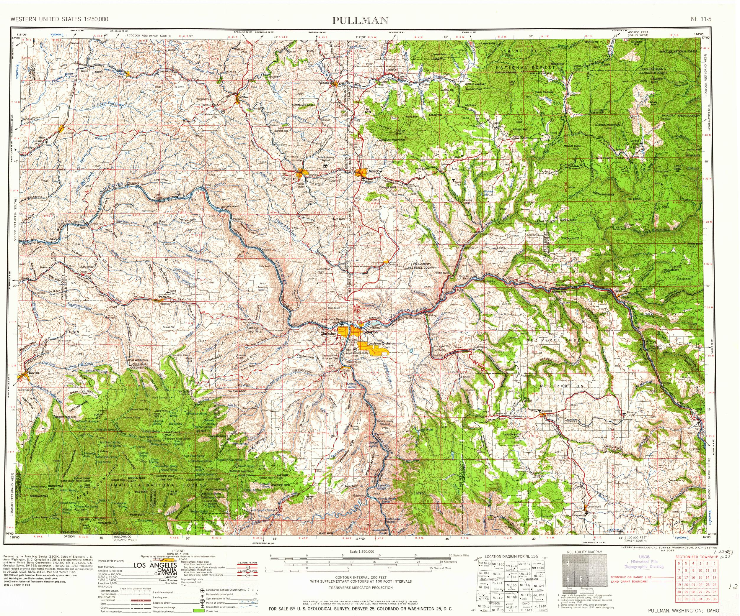
100,000-foot grids based on Idaho coordinate system, west zone and Washington coordinate system, south zone 10,000-meter Universal Transverse Mercator grid ticks, zone 11, shown in blue
