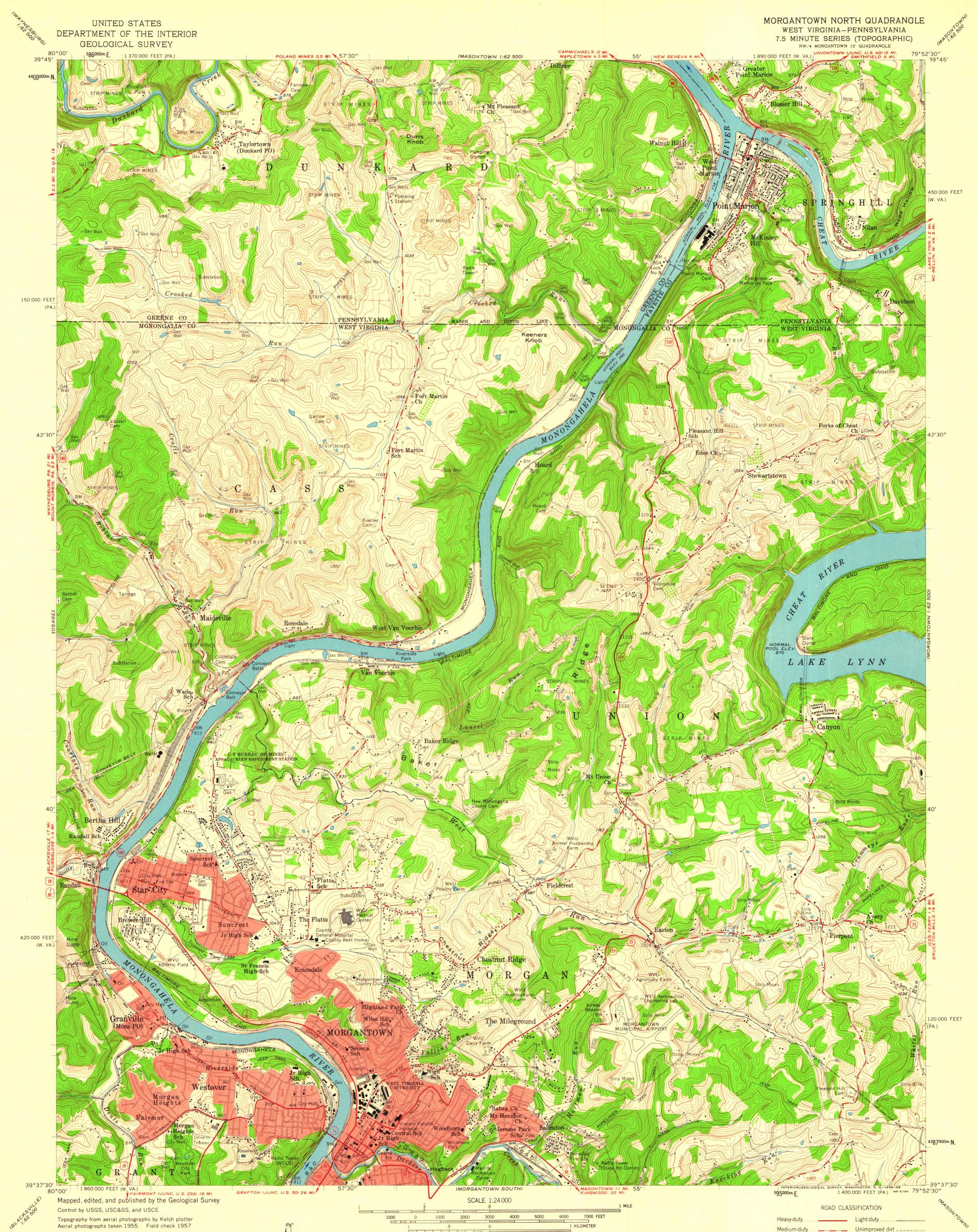
Polyconic projection. 1927 North American datum 10,000-foot grids based on West Virginia coordinate system, north zone, and Pennsylvania coordinate system, south zone 1000-meter Universal Transverse Mercator grid ticks, zone 17, shown in blue
