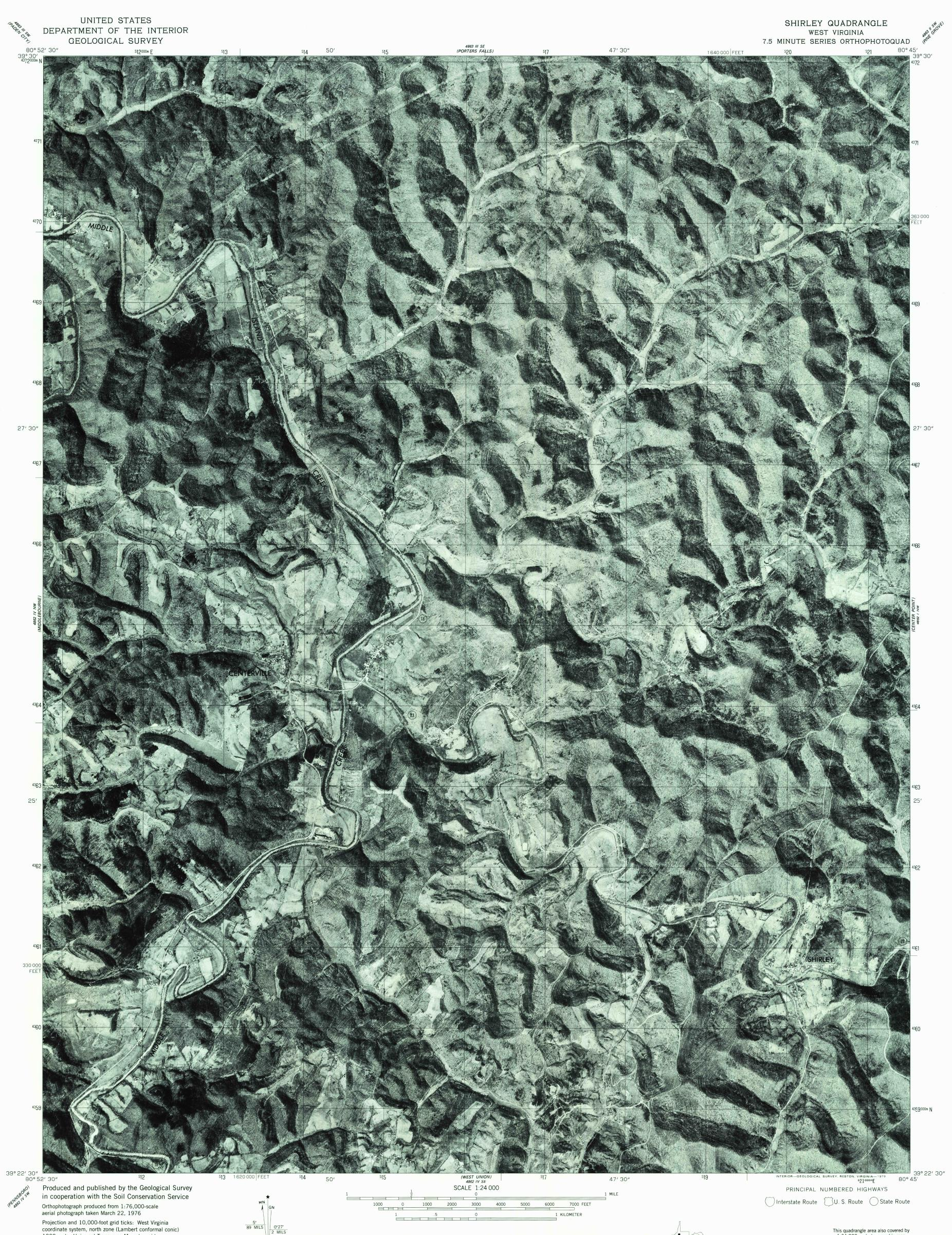
coordinate system, north zone (Lambert conformal conic) 1000-meter Universal Transverse Mercator grid, zone 17. 1927 North American datum
