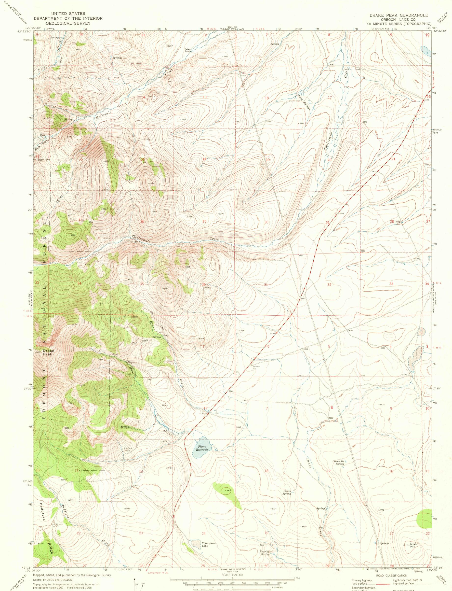
Polyconic projection. 1927 North American datum 10,000-foot grid based on Oregon coordinate system, south zone 1000-meter Universal Transverse Mercator grid ticks, zone 10, shown in blue
