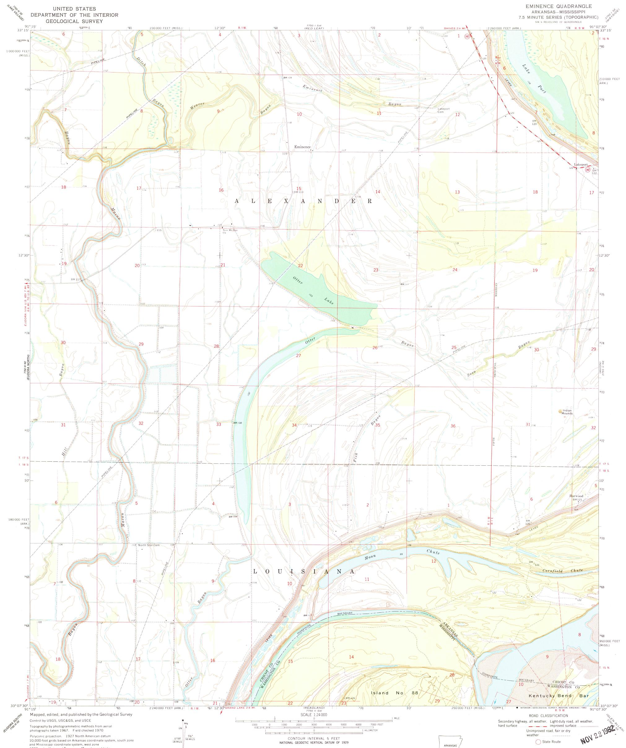
10,000-foot grids based on Arkansas coordinate system, south zone and Mississippi coordinate system, west zone 1000-meter Universal Transverse Mercator grid ticks, zone 15, shown in blue To place on the predicted North American Datum 1983 move the projection lines 11 meters south and 11 meters east as shown by dashed corner ticks Fine red dashed lines indicate selected fence and field lines where generally visible on aerial photographs. This information is unchecked
