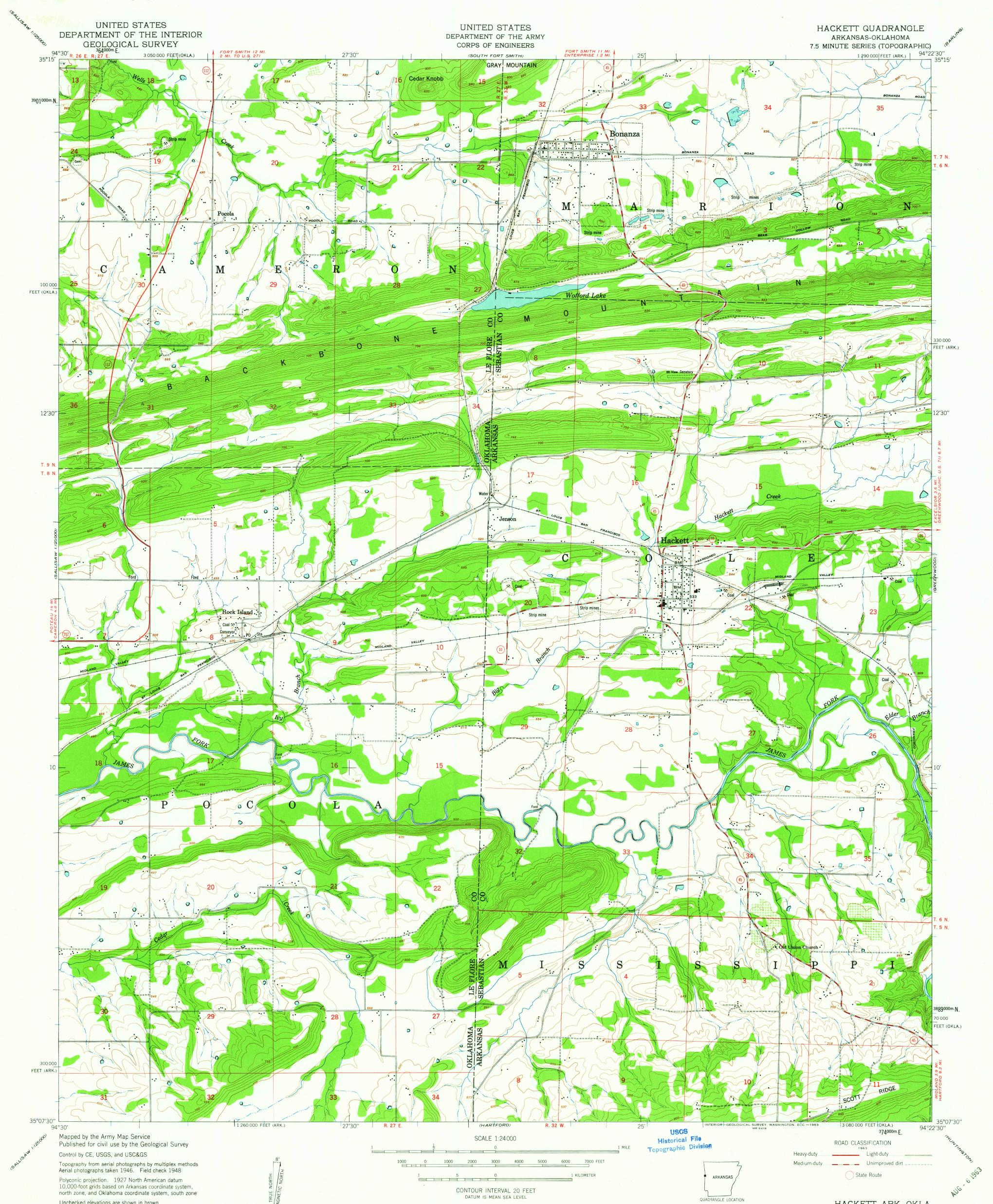
Polyconic projection. 1927 North American datum 10,000-foot grids based on Arkansas coordinate system, north zone, and Oklahoma coordinate system, south zone
