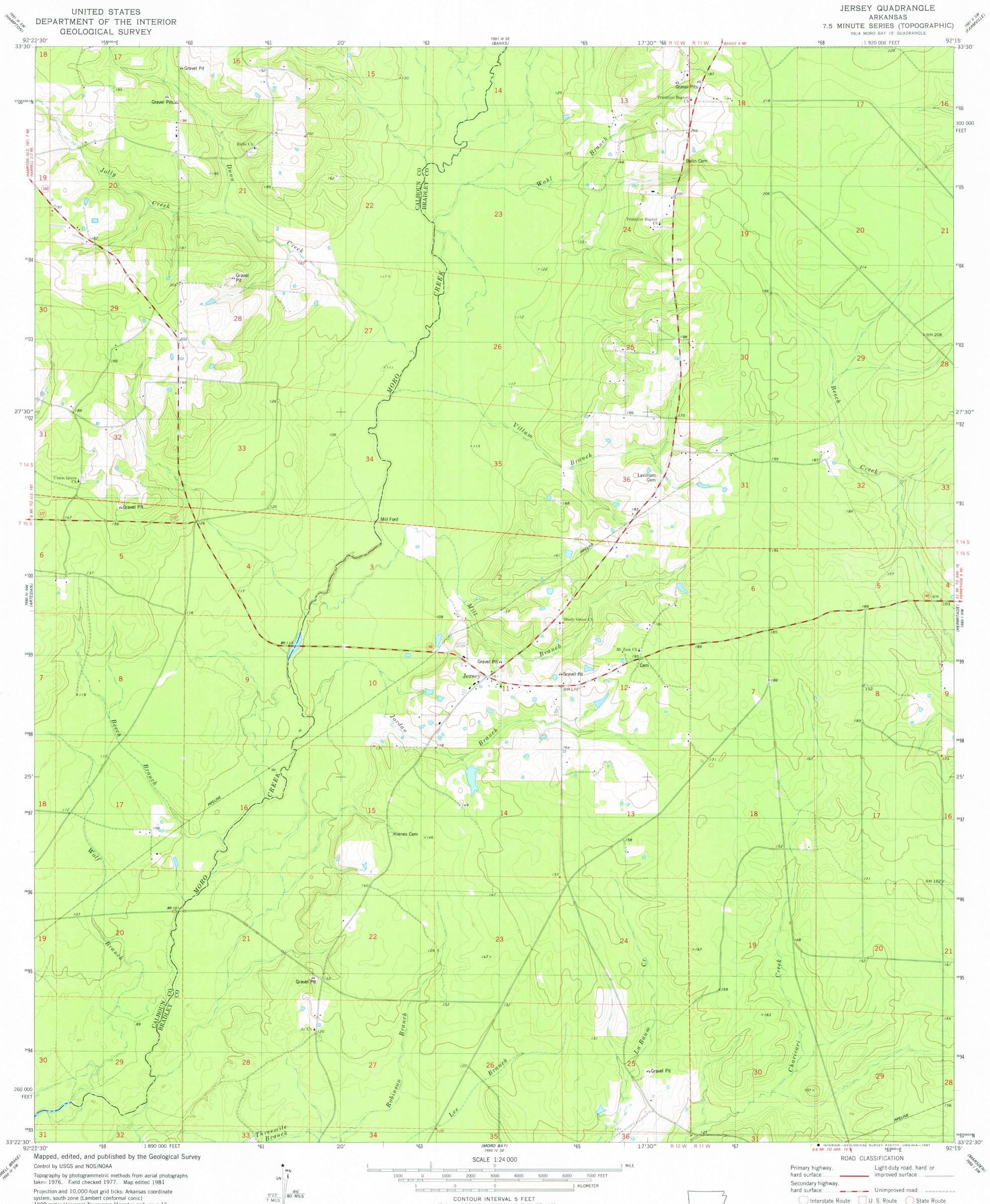
system, south zone (Lambert conformal conic) 1000-meter Universal Transverse Mercator grid, zone 15 1927 North American Datum To place on the predicted North American Datum 1983 move the projection lines 10 meters south and 14 meters east as shown by dashed corner ticks
