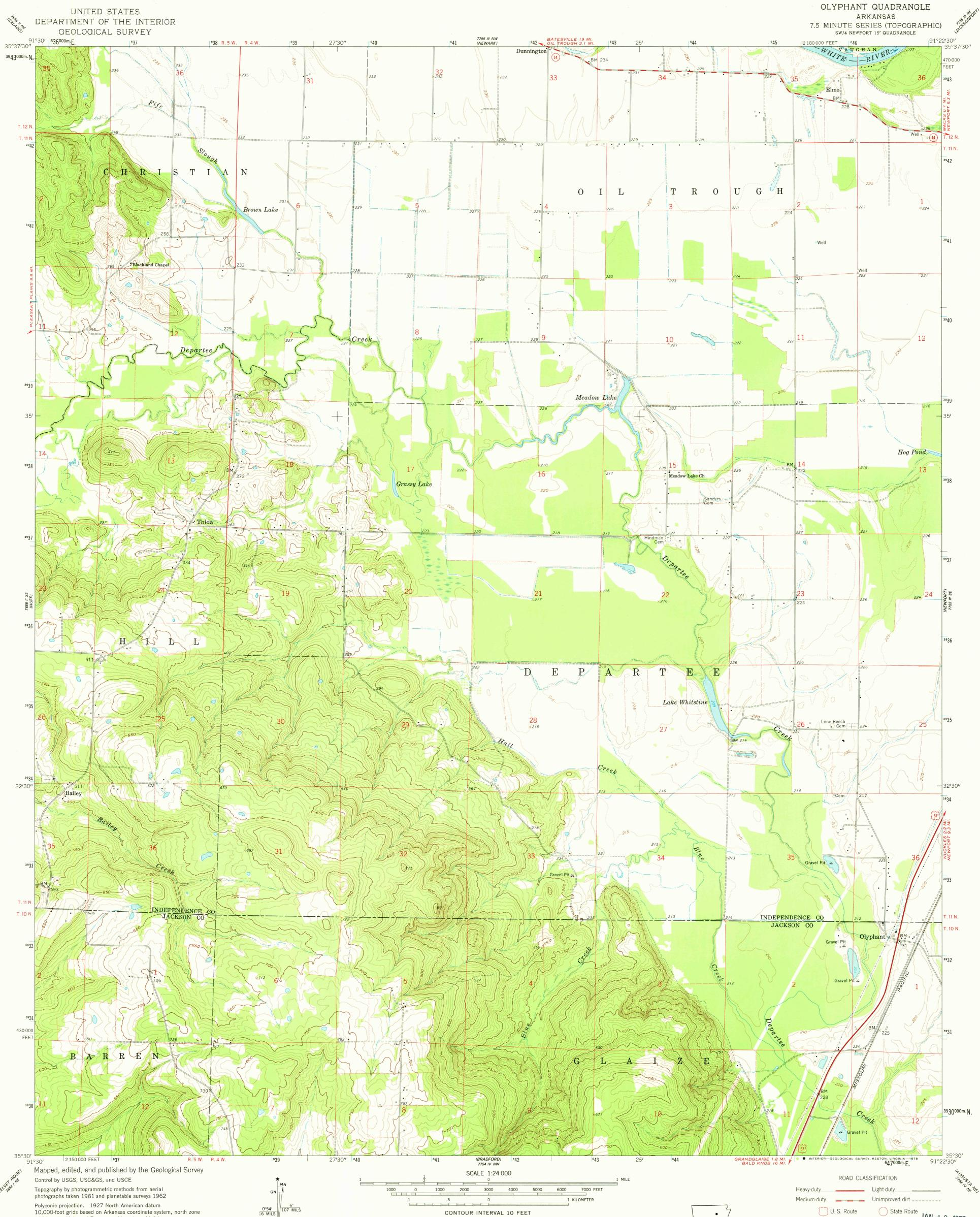
10,000-foot grids based on Arkansas coordinate system, north zone 1000-meter Universal Transverse Mercator grid ticks, zone 15, shown in blue
