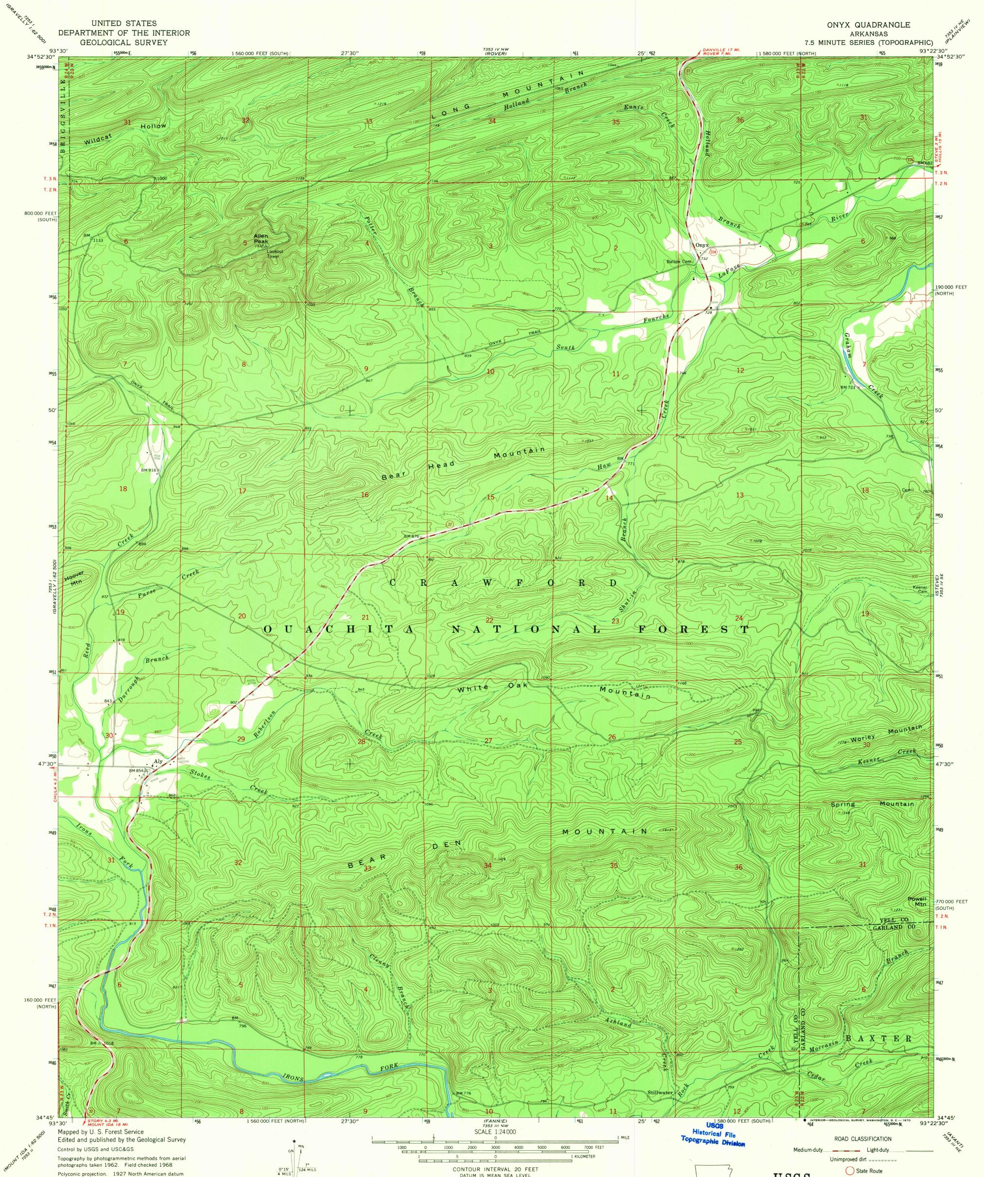
Polyconic projection. 1927 North American datum 10,000-foot grids based on Arkansas coordinate system, north and south zones 1000-meter Universal Transverse Mercator grid ticks, zone 15, shown in <mark>b</mark>lue
