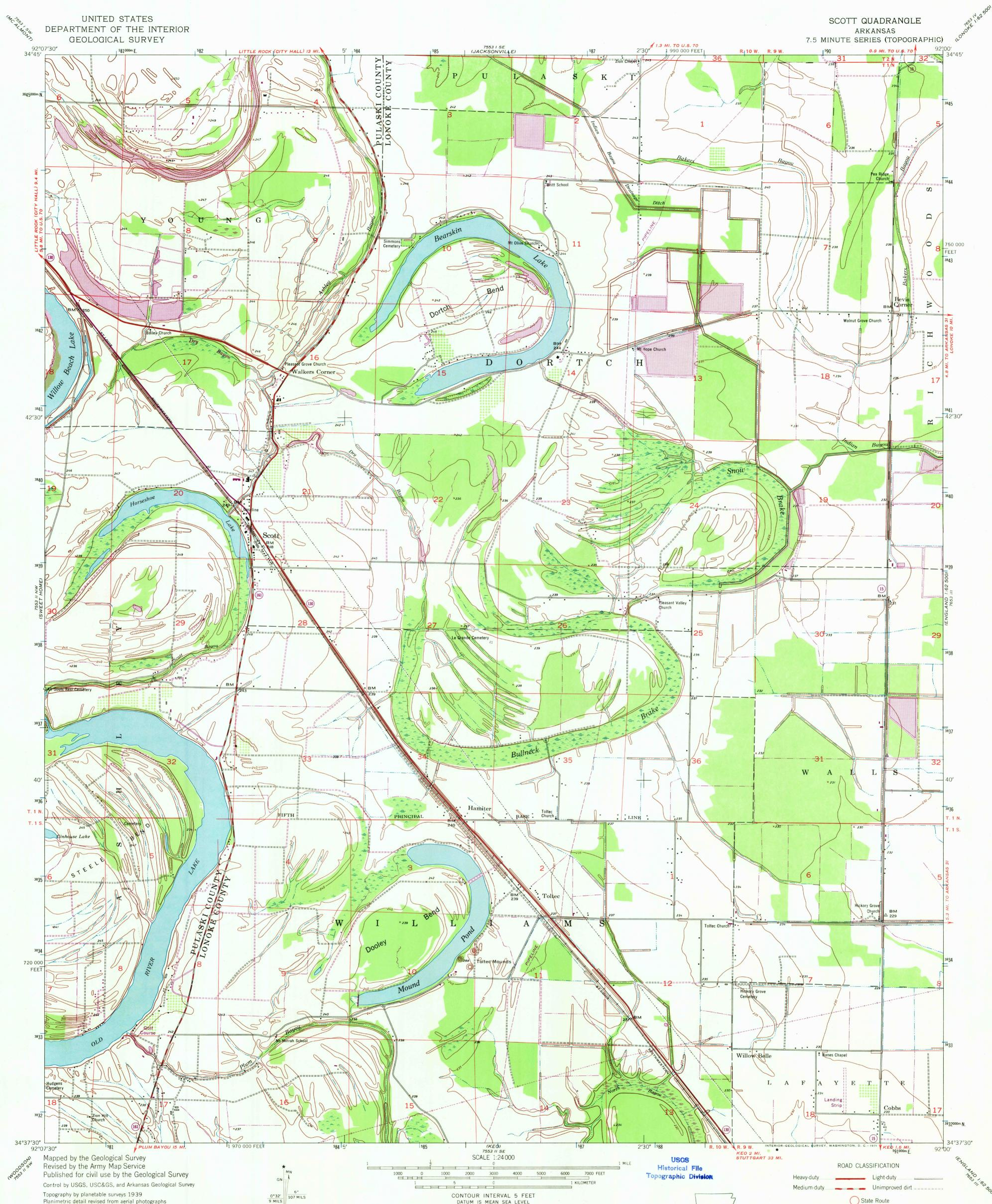
Topography by planetable surveys 1939 Planimetric detail revised from aerial photographs taken 1952. Field check 1954
