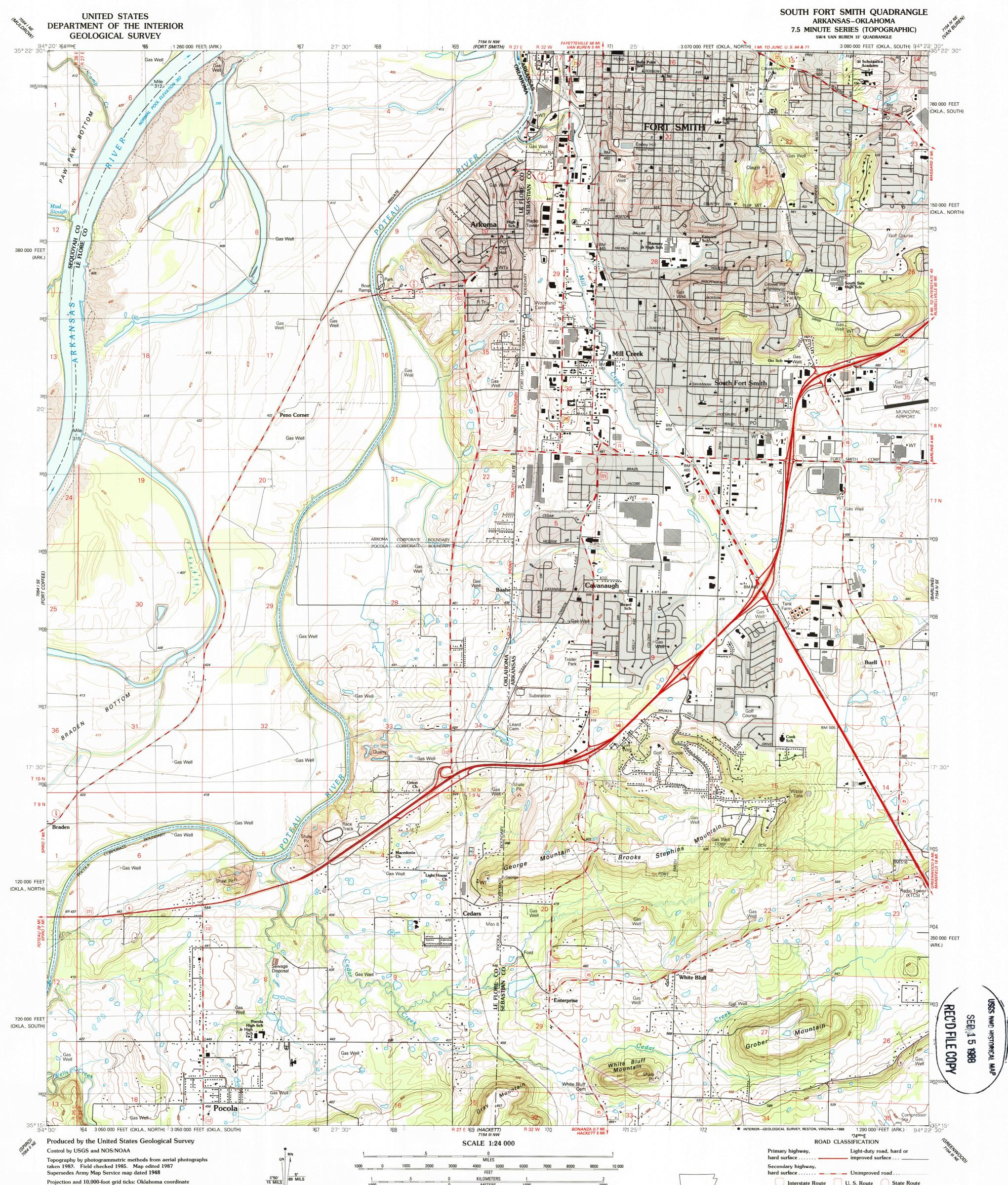
Projection and 10,000-foot grid ticks: Oklahoma coordinate system, south and north zones, and Arkansas coordinate system, north zone (Lambert conformal conic) 1000-meter Universal Transverse Mercator grid, zone 15 1927 North American Datum To place on the predicted North American Datum 1983, move the projection lines 6 meters south and 19 meters east as shown by dashed corner ticks There may be private inholdings within the boundaries of
