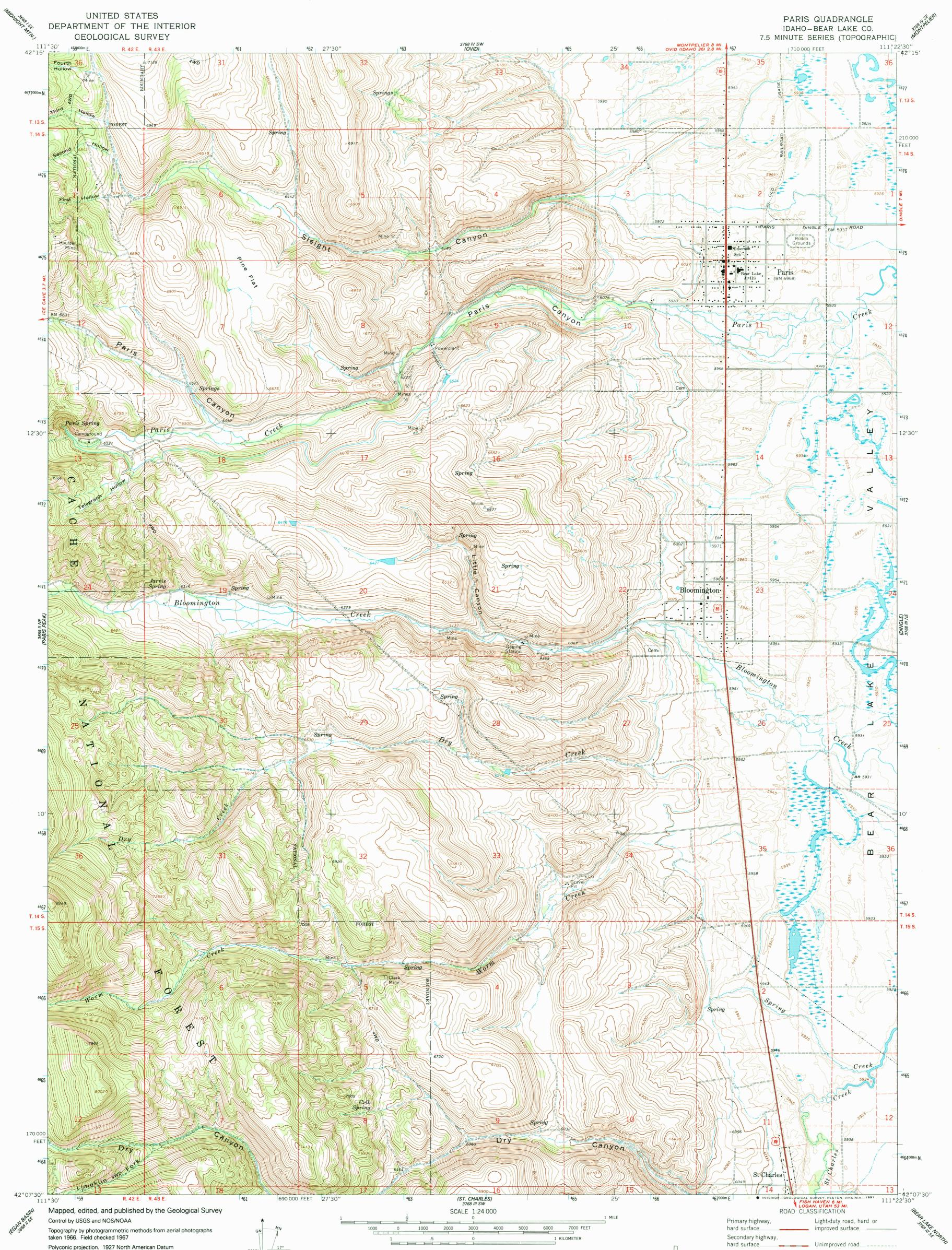
0°18' 5 MILS /302 MILS 10,000-foot grid based on Idaho coordinate system, east zone 1000-meter Universal Transverse Mercator grid ticks, zone 12, shown in blue The difference between 1927 North American Datum and North UTM GRID AND 1967 MAGNETIC NORTH DECLINATION AT CENTER OF SHEET American Datum of 1983 (NAD 83) for 7.5 minute intersections is given in USGS Bulletin 1875. The NAD 83 is shown by dashed corner ticks Fine red dashed lines indicate selected fence lines
