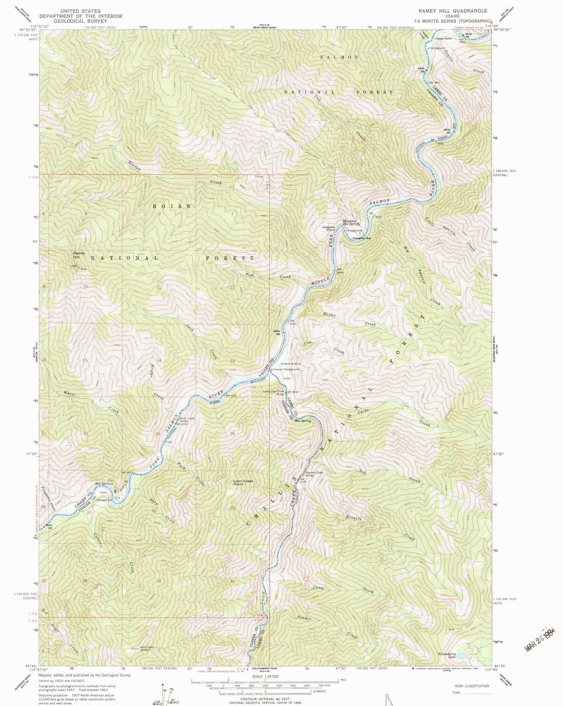
central and west zones 1000-meter Universal Transverse Mercator grid ticks, zone 11, shown in blue To place on the predicted North American Datum 1983 move the projection lines 14 meters north and 73 meters east as shown by dashed corner ticks Where omitted, land lines have not been established There may be private inholdings within the boundaries of
