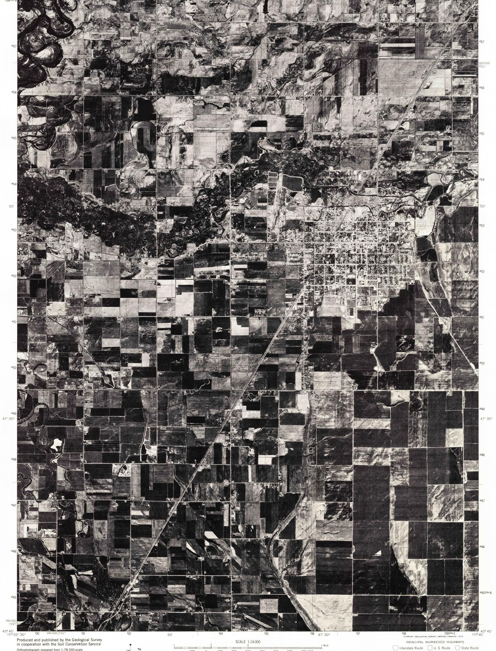
Produced and published by the Geological Survey in cooperation with the Soil Conservation Service Orthophotograph prepared from 1:78 000-scale aerial photographs taken August 5, 1976 Projection and 10,000—foot grid ticks: Idaho coordinate system, east zone (transverse Mercator) 1000-meter Universal Transverse Mercator grid ticks, zone 12. 1927 North American datum
