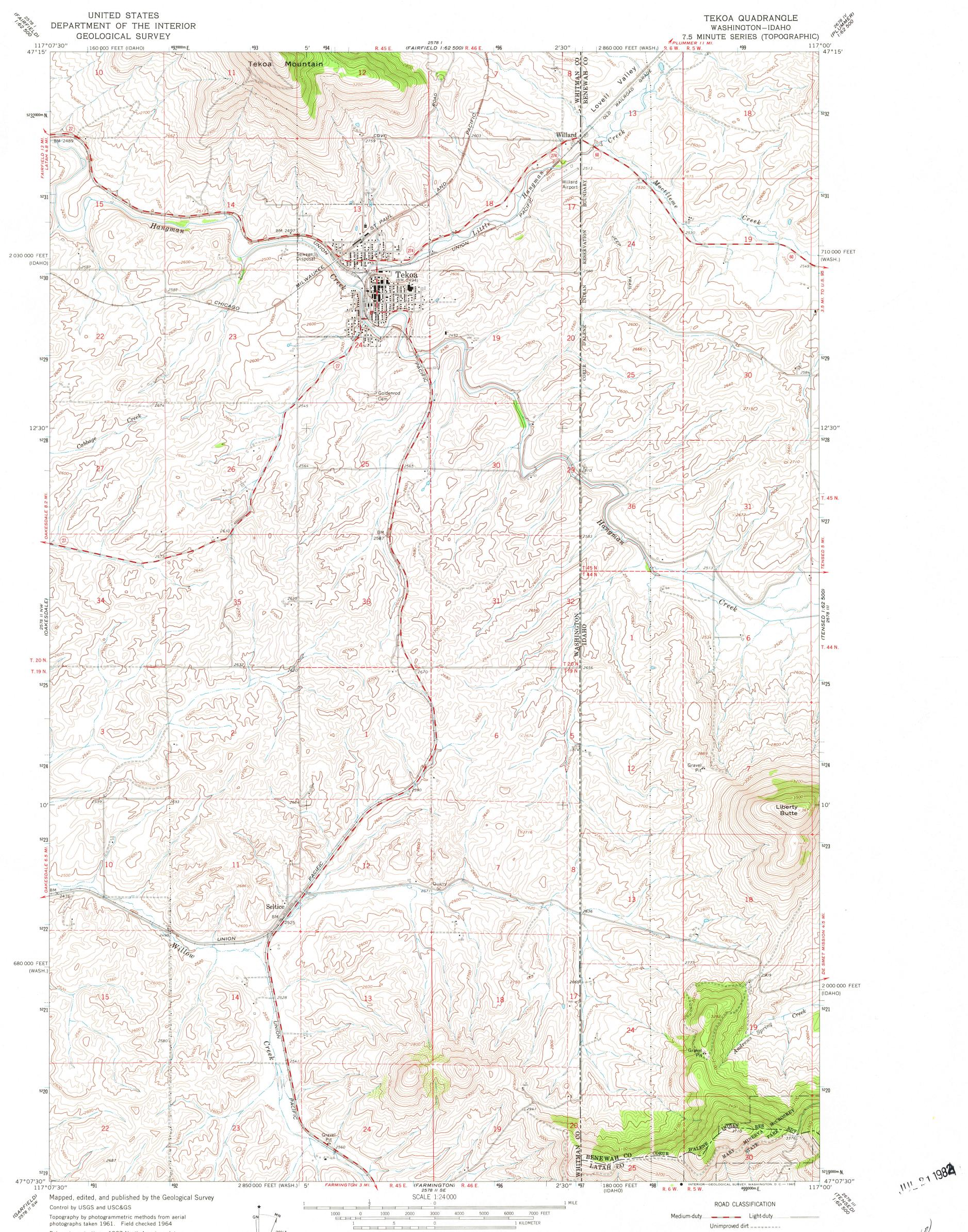
Polyconic projection. 1927 North American datum 10,000-foot grids based on Washington coordinate system, south zone, and Idaho coordinate system, west zone 1000-meter Universal Transverse Mercator grid ticks, zone 11, shown in blue UTM GRID AND 1964 MAGNETIC NORTH DECLINATION AT CENTER OF SHEET
