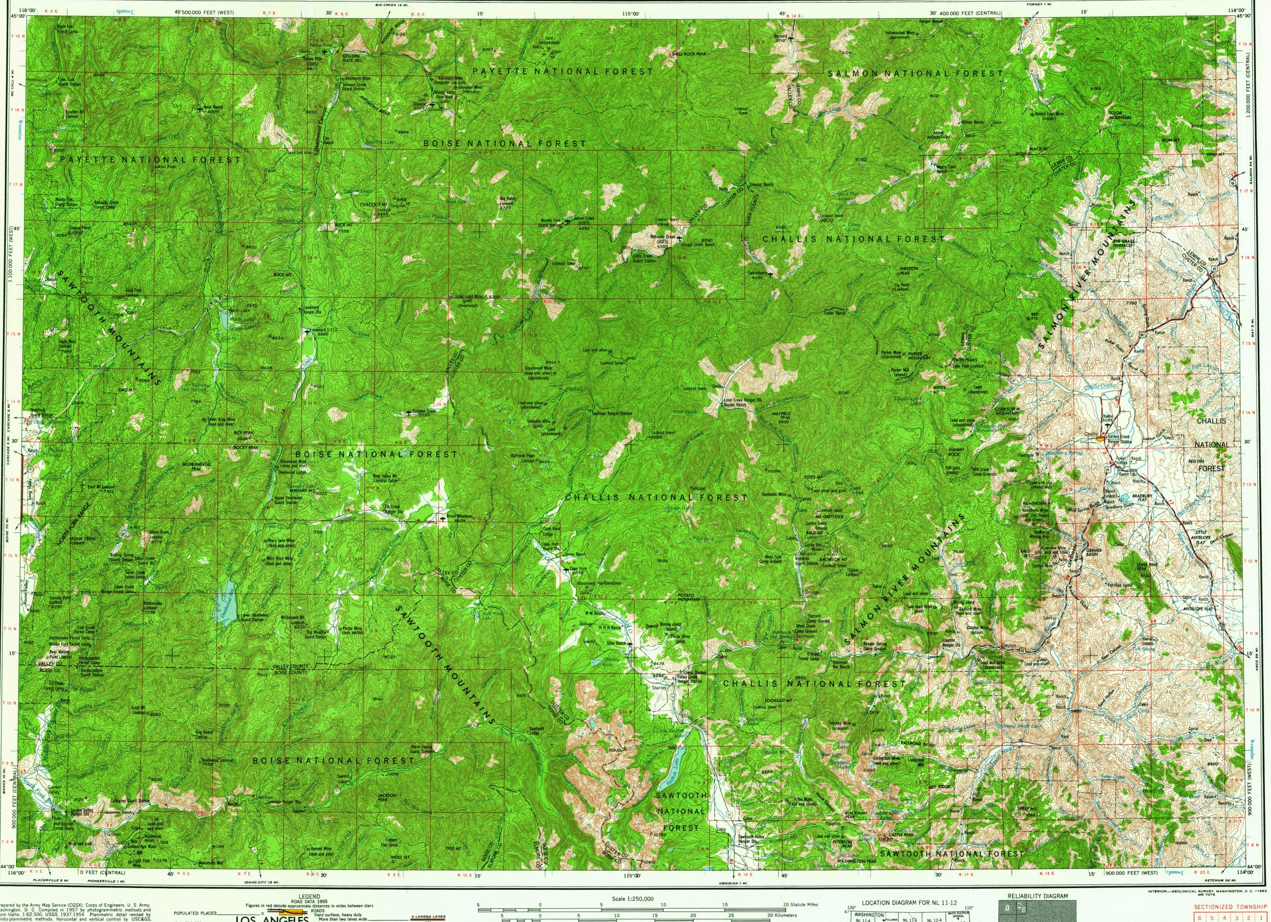
Prepared by the Army Map Service (CGSX), Corps of Engineers, U. S. Army, Washington, D. C. Compiled in 1957 by photogrammetric methods and from Idaho, 1:62,500, USGS, 1937-1954. Planimetric detail revised by photo-planimetric methods. Horizontal and vertical control by USC&GS, USGS and CE. Photography field annotated 1955. 100,000-foot grids based on Idaho coordinate system,
