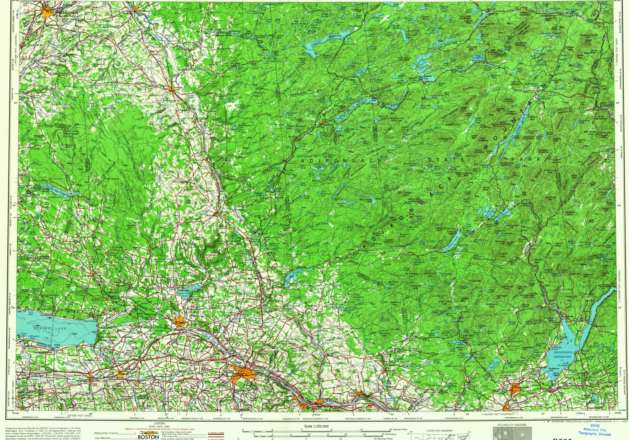
Prepared by the Army Map Service (KCGE), Corps of Engineers, U.S. Army, Washington, D.C. Compiled in 1961 by photogrammetric methods and from: United States Quadrangles, 1:24,000, 1:25,000, 1:62,500, U.S. Geological Survey and AMS, 1940-59. Planimetric detail revised by photoplanimetric methods. Horizontal and vertical control by USGS, USC&GS, TVA, and New York Geodetic Survey. Map field checked 1962.
