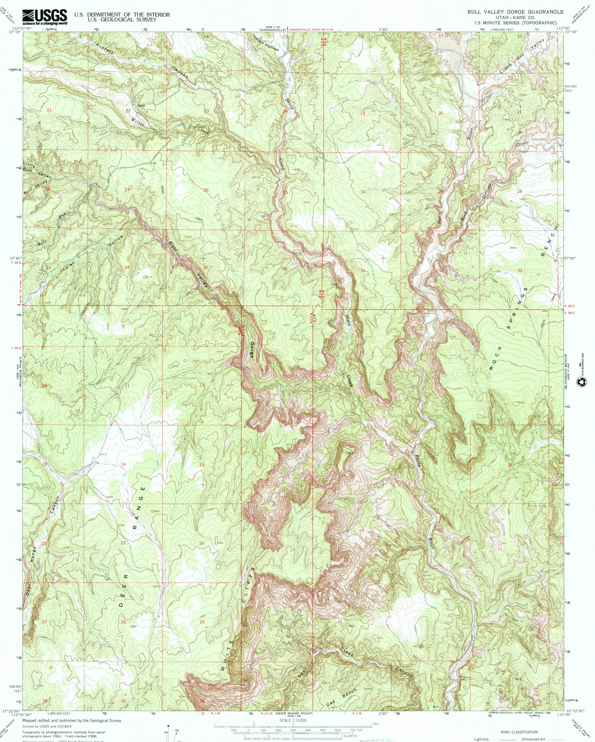
Polyconic projection. 1927 North American datum 10,000-foot grid based on Utah coordinate system, south zone 1000-meter Universal Transverse Mercator grid ticks, zone 12, shown in blue
