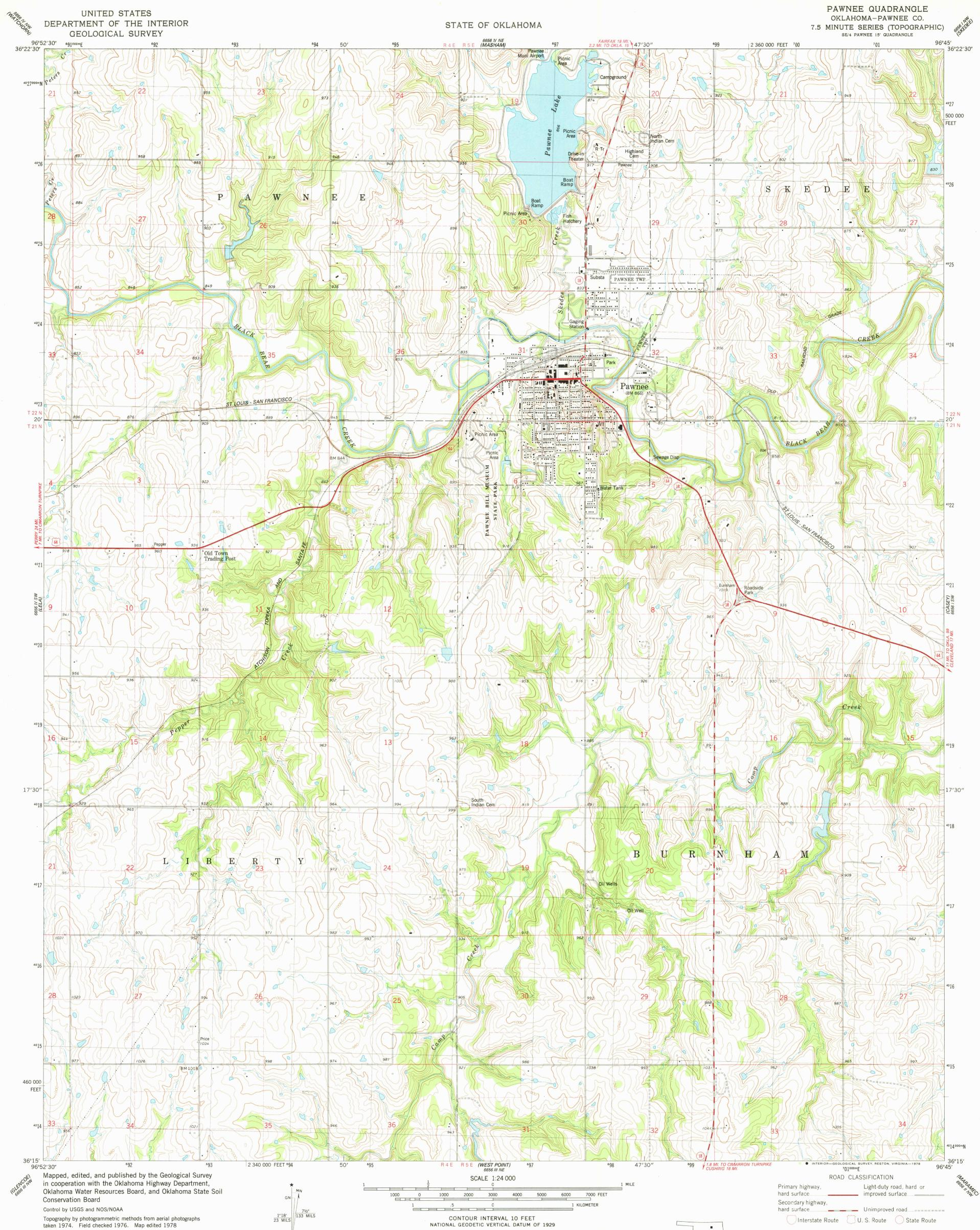
Projection and 10,000-foot grid ticks: Oklahoma coordinate system, north zone (Lambert conformal conic) 1000-meter Universal Transverse Mercator grid, zone 14 1927 North American datum
