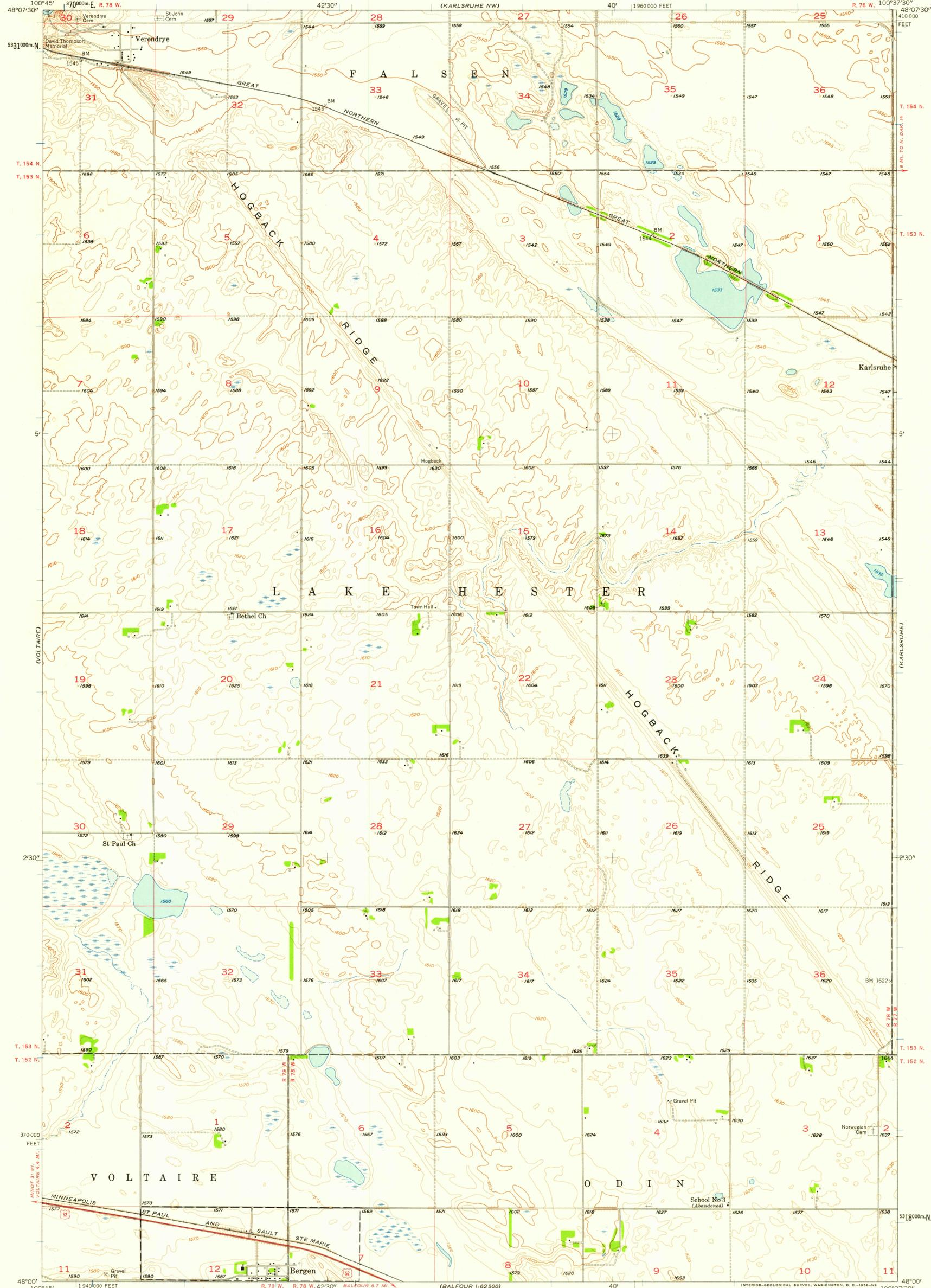
Mapped, edited, and published by the Geological Survey as part of the Department of the Interior program for the development of the Missouri River Basin. Control by USGS and USC&GS. Topography from aerial photographs by photogrammetric methods. Aerial photographs taken 1956. Field check 1957. Polyconic projection. 1927 North American datum. 10,000-foot grid based on North Dakota coordinate system, north zone. 1000-meter Universal Transverse Mercator grid ticks, zone 14, shown in blue.
