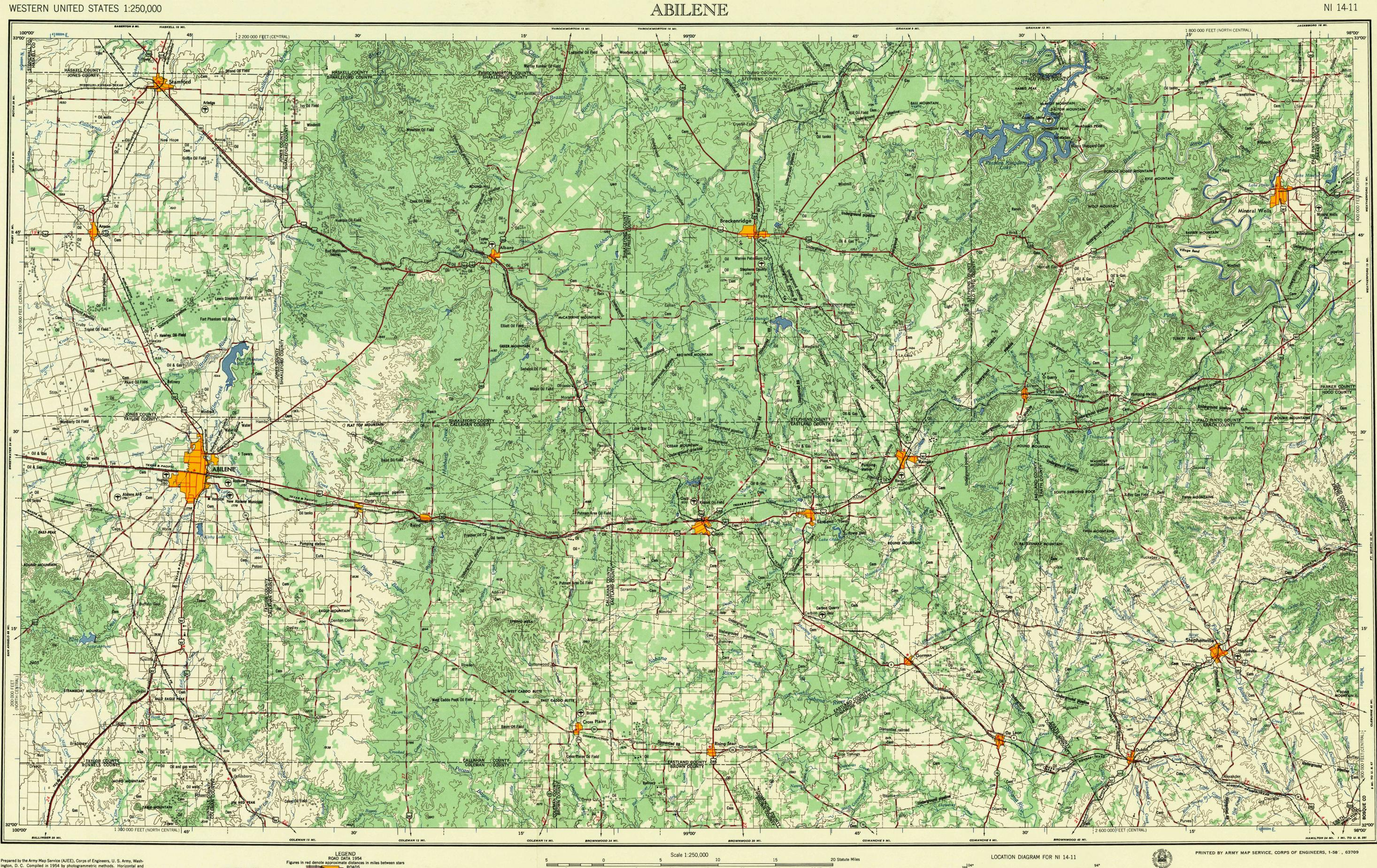
Prepared by the Army Map Service (AJEE), Corps of Engineers, U. S. Army, Wash-ington, D. C. Compiled in 1954 by photogrammetric methods. Horizontal and vertical control by USC&GS and USGS. Aerial photography 1952–53. Photog-raphy field annotated 1954. 100,000 foot grids based on Texas coordinate system, north central and central zones 10,000-meter Universal Transverse Mercator grid ticks, zone 14, shown in blue
