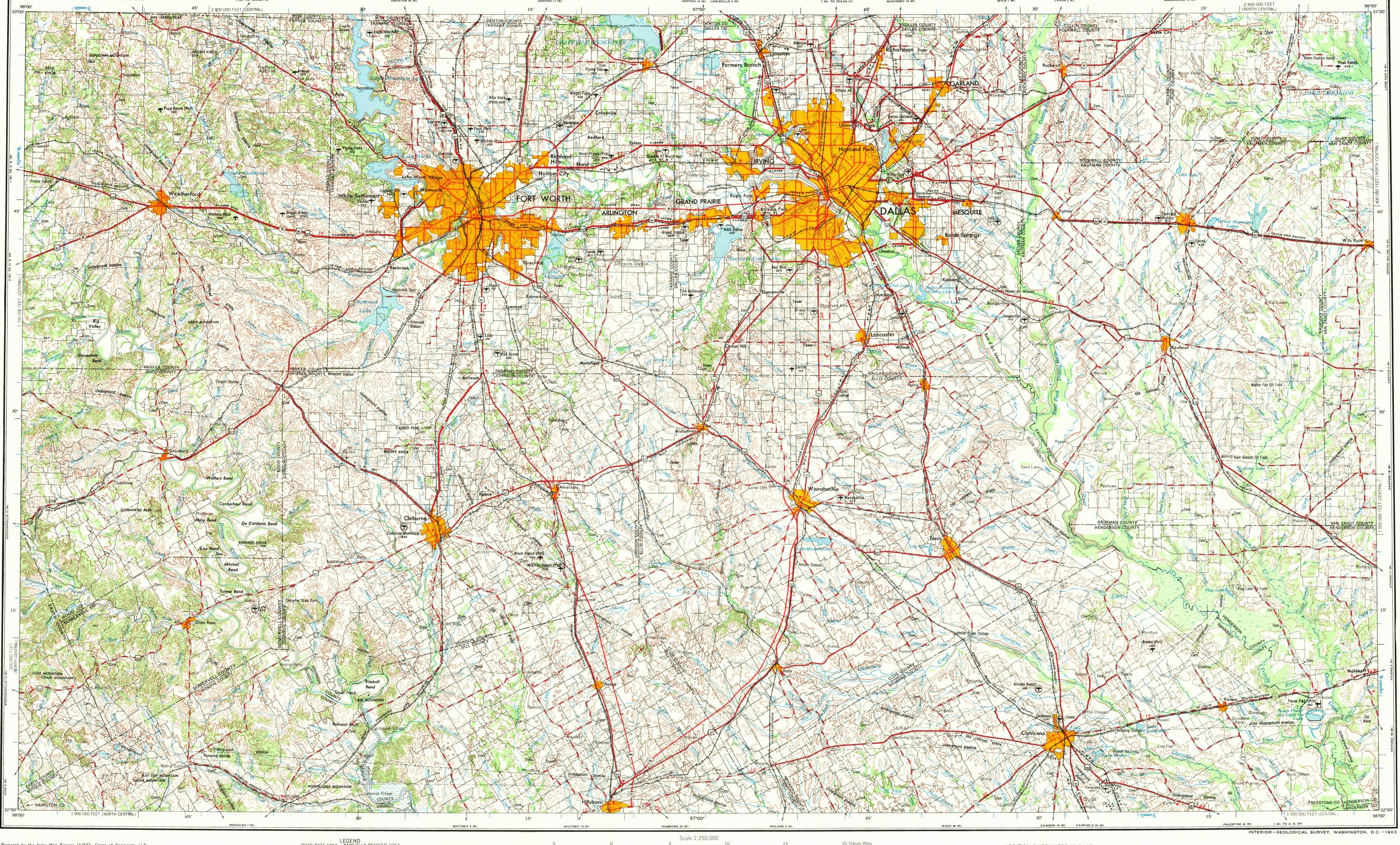
Prepared by the Army Map Service (AJEE), Corps of Engineers, U.S. Army, Washington, D.C. Compiled in 1954 by photogrammetric methods. Horizontal and vertical control by USGS and USC&GS. Aerial photography 1952-53. Photography field annotated 1954. Limited revision by U.S. Geological Survey 1963
