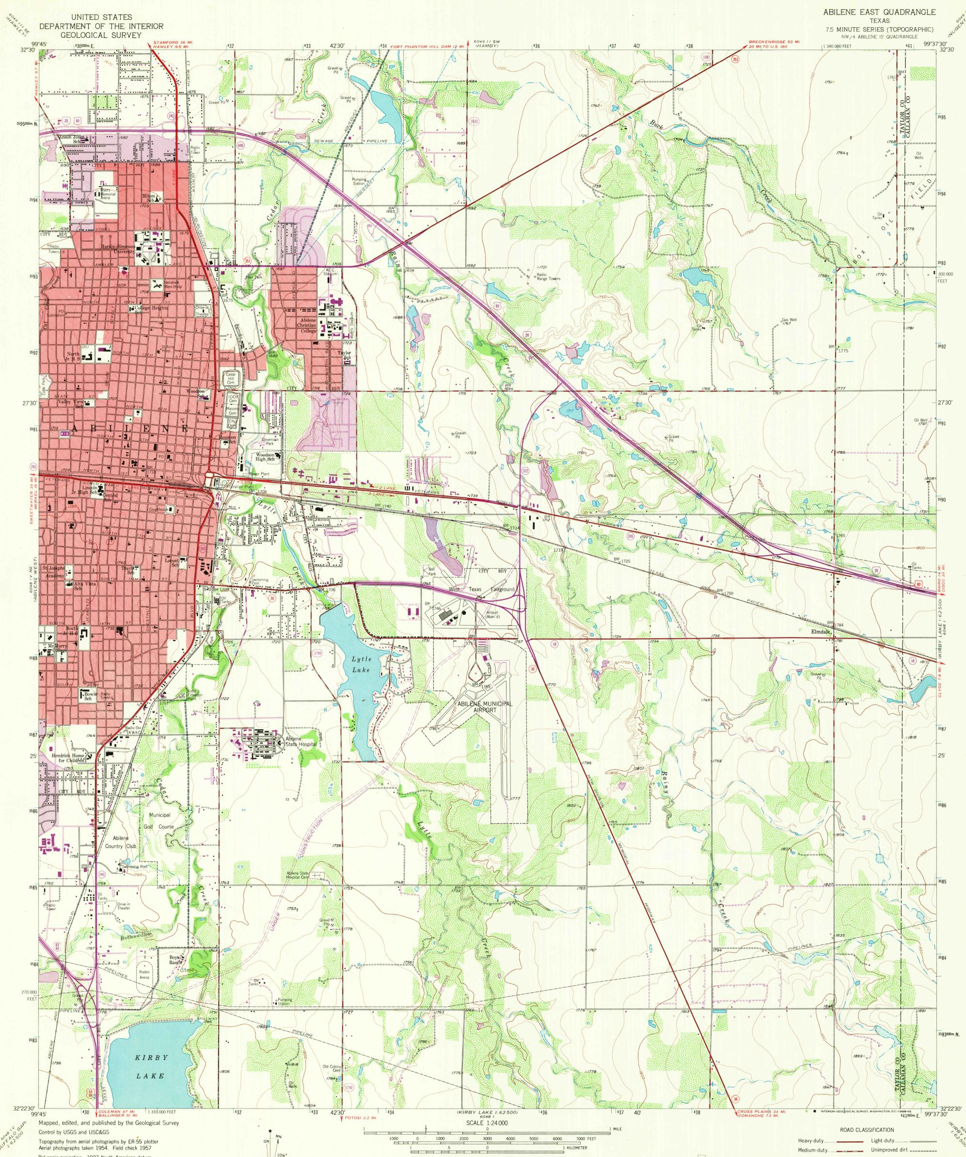
Polyconic projection. 1927 North American datum 10,000-foot grid based on Texas coordinate system, north central zone 1000-meter Universal Transverse Mercator grid ticks, zone 14, shown in blue
