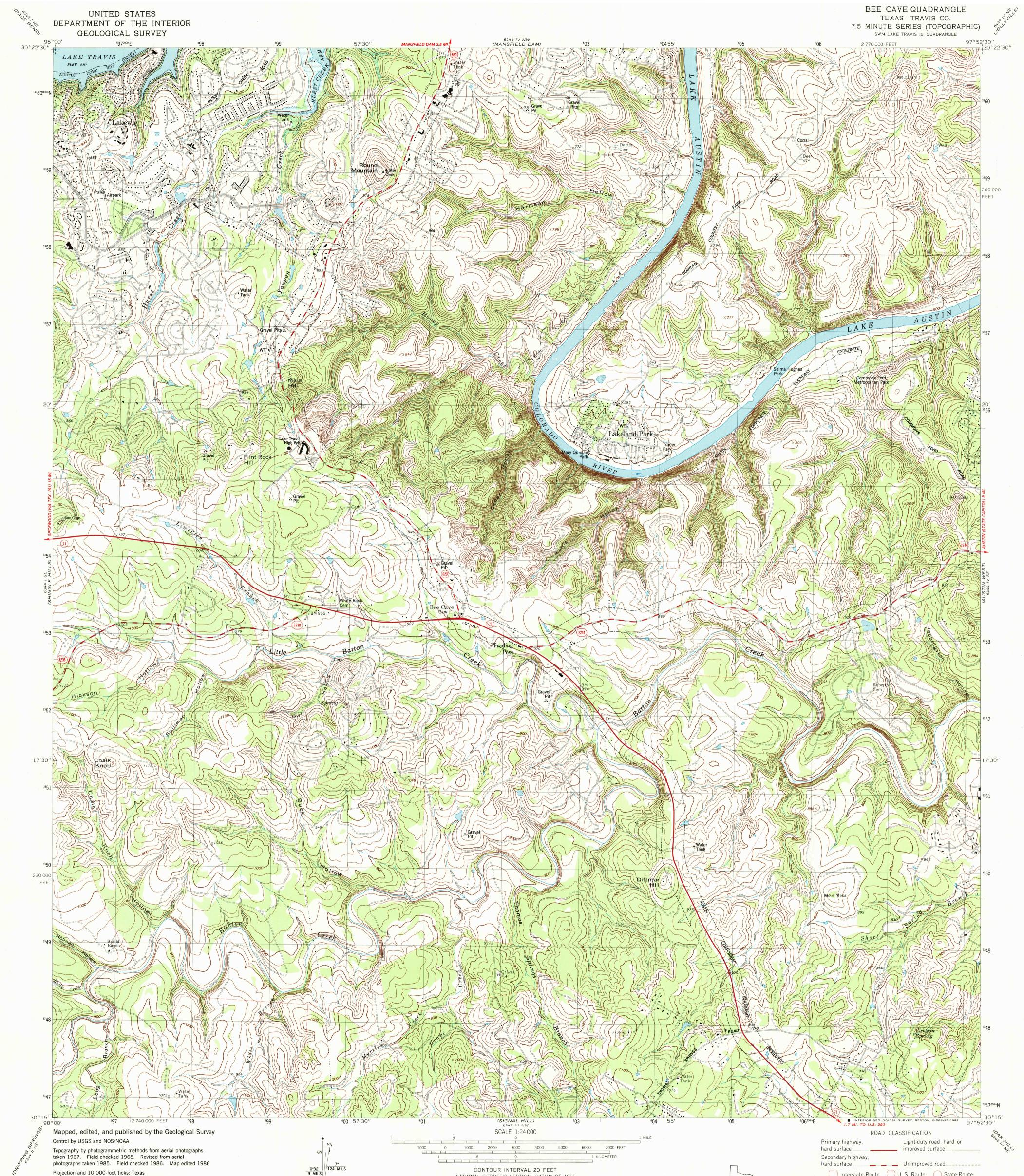
Projection and 10,000-foot ticks: Texas coordinate system, central zone (Lambert conformal conic) 1000-meter Universal Transverse Mercator grid, zone 14 1927 North American Datum To place on the predicted North American Datum 1983 move the projection lines 18 meters south and 28 meters east as shown by dashed corner ticks
