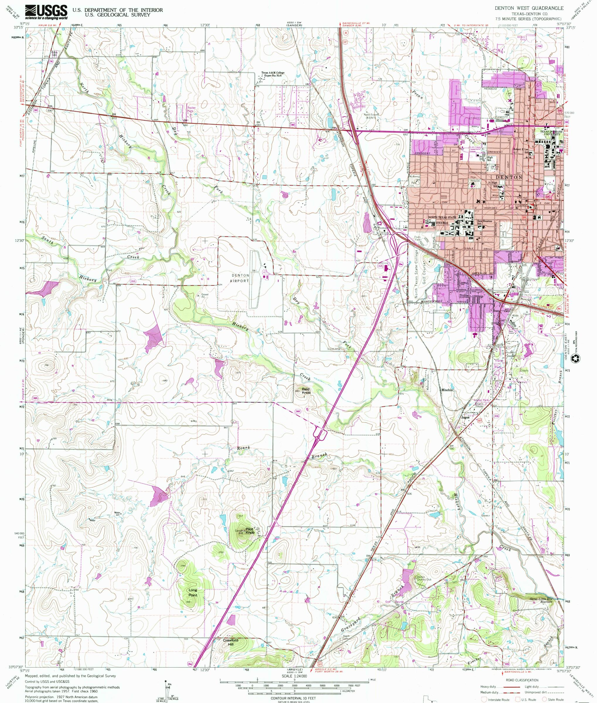
10,000 foot grid based on Texas coordinate system, north central zone 1000-meter Universal Transverse Mercator grid ticks,
