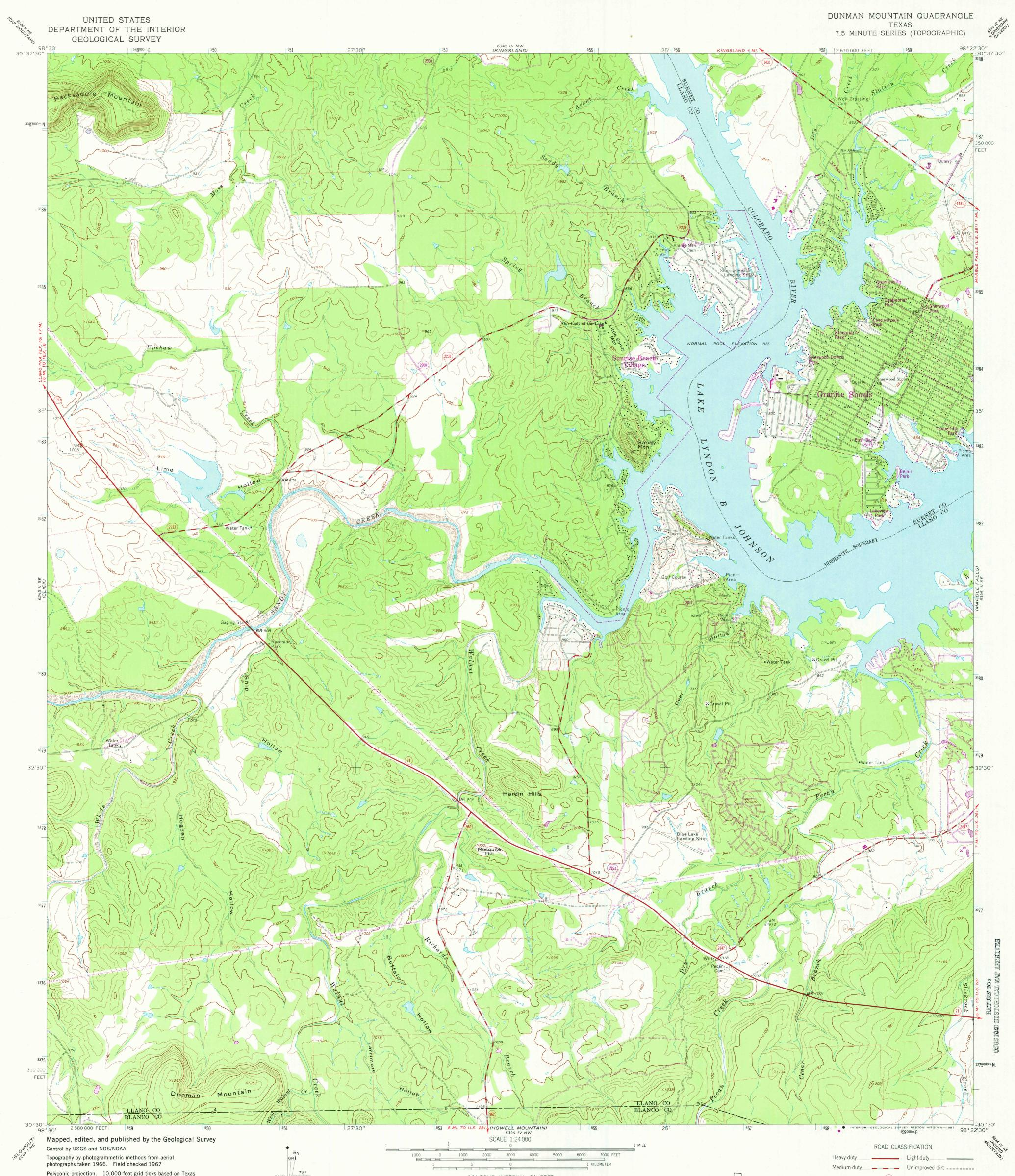
coordinate system, central zone. 1000-meter Universal Transverse Mercator grid ticks, zone 14, shown in blue. 1927 North American Datum. To place on the predicted North American Datum 1983 move the projection lines 17 meters south and 30 meters east as shown by dashed corner ticks Fine red dashed lines indicate selected fence lines
