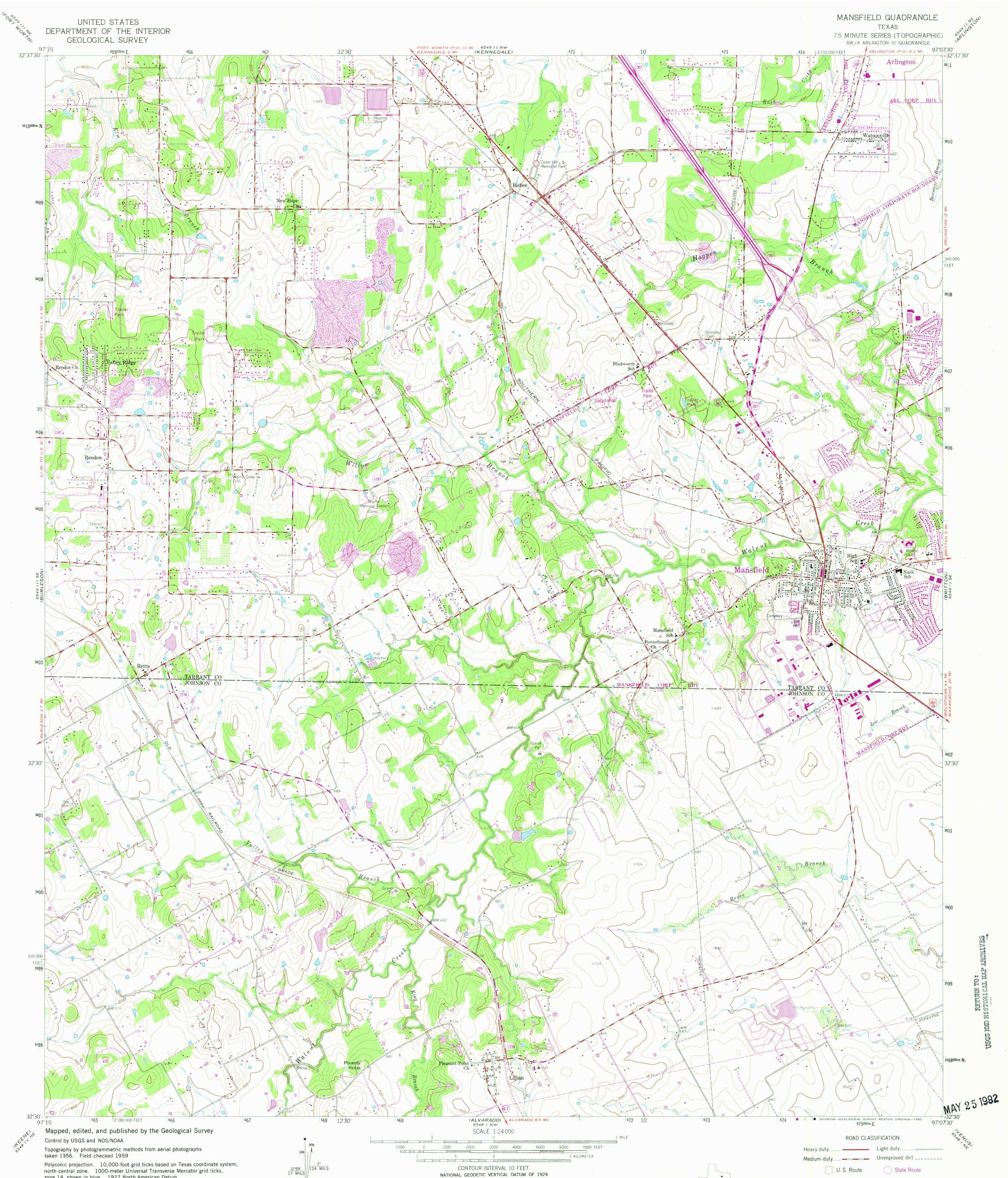
Polyconic projection. 10,000-foot grid ticks based on Texas coordinate system, north central zone. 1000-meter Universal Transverse Mercator grid ticks, zone 14, shown in blue. 1927 North American Datum To place on the predicted North American Datum 1983 move the projection lines 11 meters south and 27 meters east as shown by dashed corner ticks
