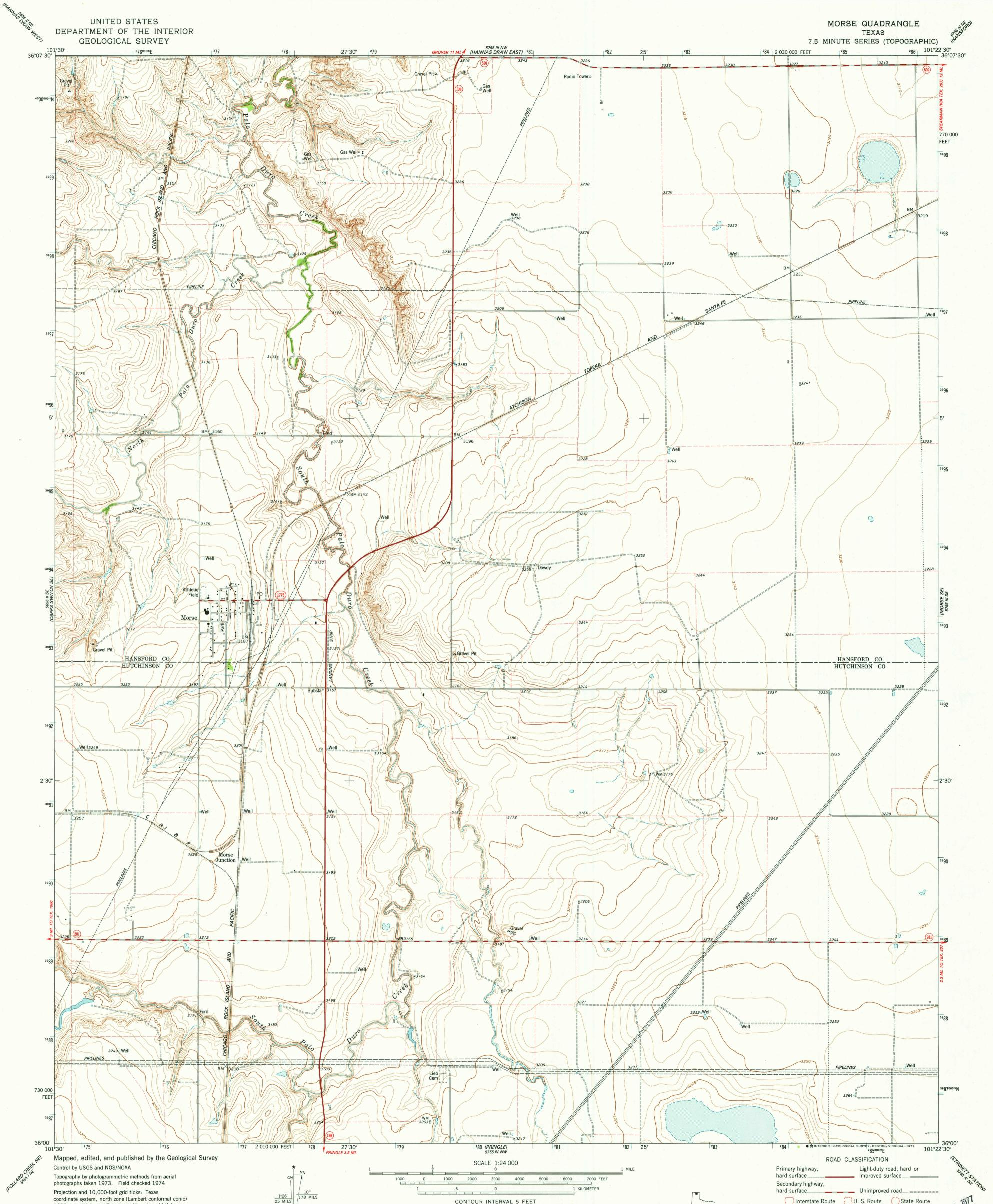
Projection and 10,000-foot grid ticks: Texas coordinate system, north zone (Lambert conformal conic) 1000-meter Universal Transverse Mercator grid ticks zone 14, shown in blue. 1927 North American datum Fine red dashed lines indicate selected fence lines
