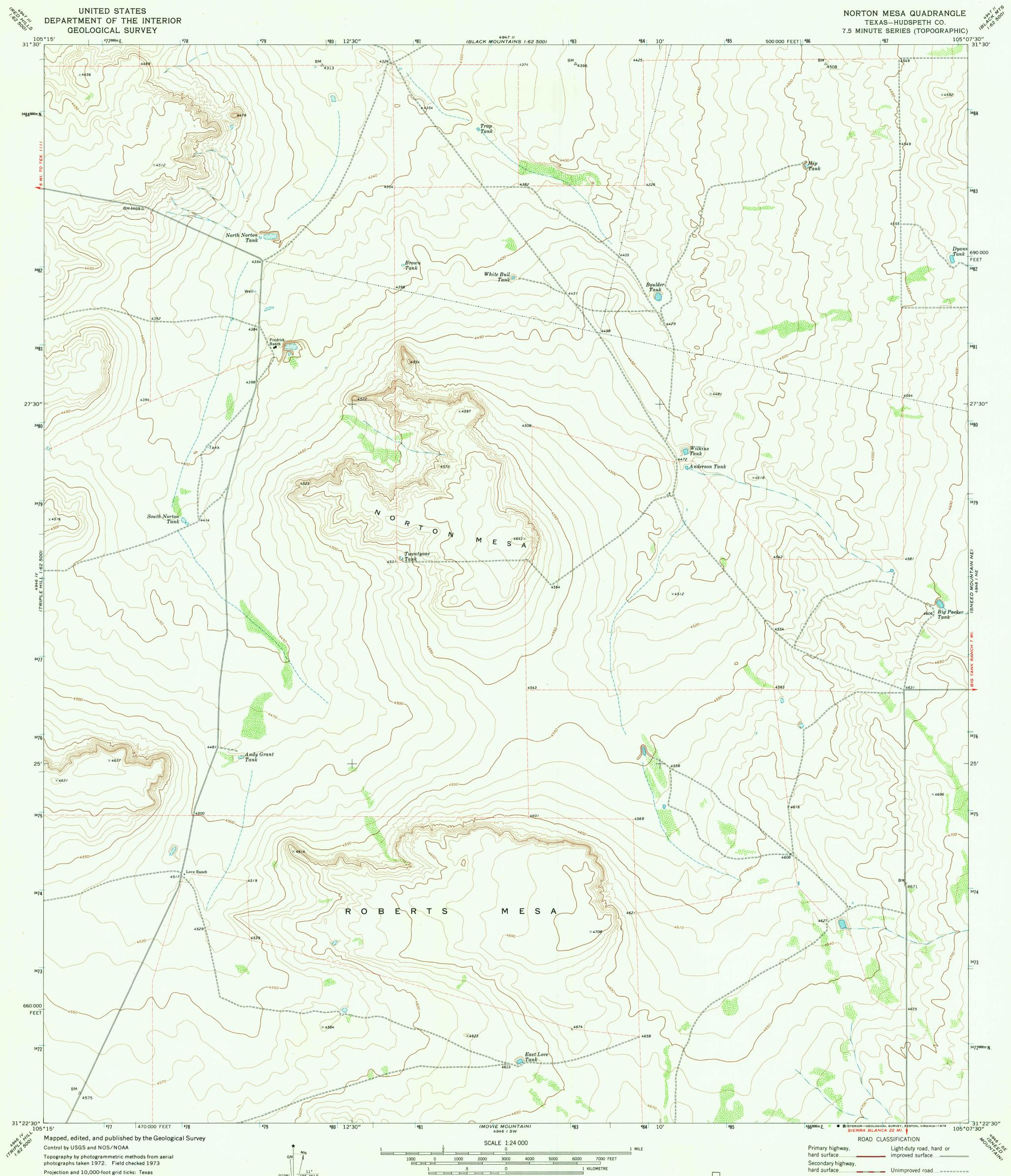
coordinate system, central zone (Lambert conformal conic) 1000-metre Universal Transverse Mercator grid ticks, zone 13, shown in blue. 1927 North American datum
