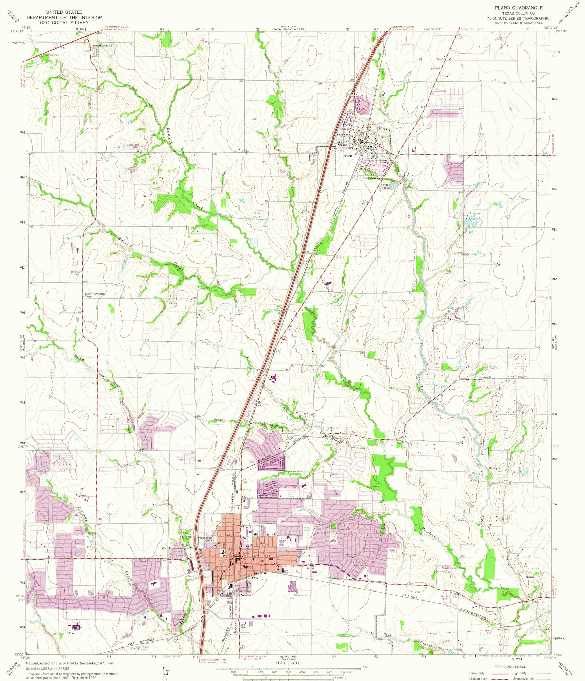
Polyconic projection. 1927 North American datum 10,000 foot grid based on Texas coordinate system, north central zone 1000-meter Universal Transverse Mercator grid ticks, zone 14, shown in blue Red tint indicates area in which only landmark buildings are shown Fine red dashed lines indicate selected force and field lines
