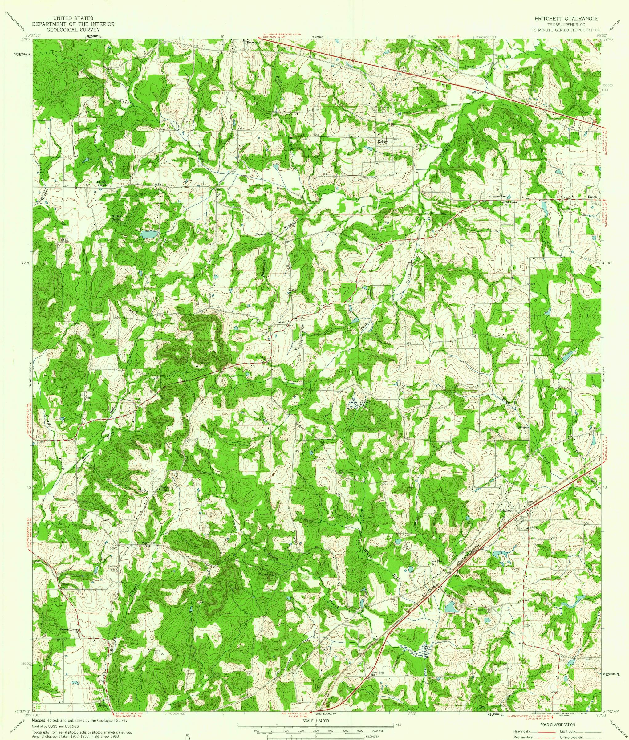
Polyconic projection. 1927 North American datum 10,000-foot grid based on Texas coordinate system, north central zone 1000-meter Universal Transverse Mercator grid ticks, zone 15, shown in blue NORTH CONTOUR INTERVAL 10 FEET DATUM IS MEAN SEA LEVEL TIC Fine red dashed lines indicate selected fence and field lines where generally visible on aerial photographs This information is unchecked APPROXIMATE MEAN DECLINATION, 1960
