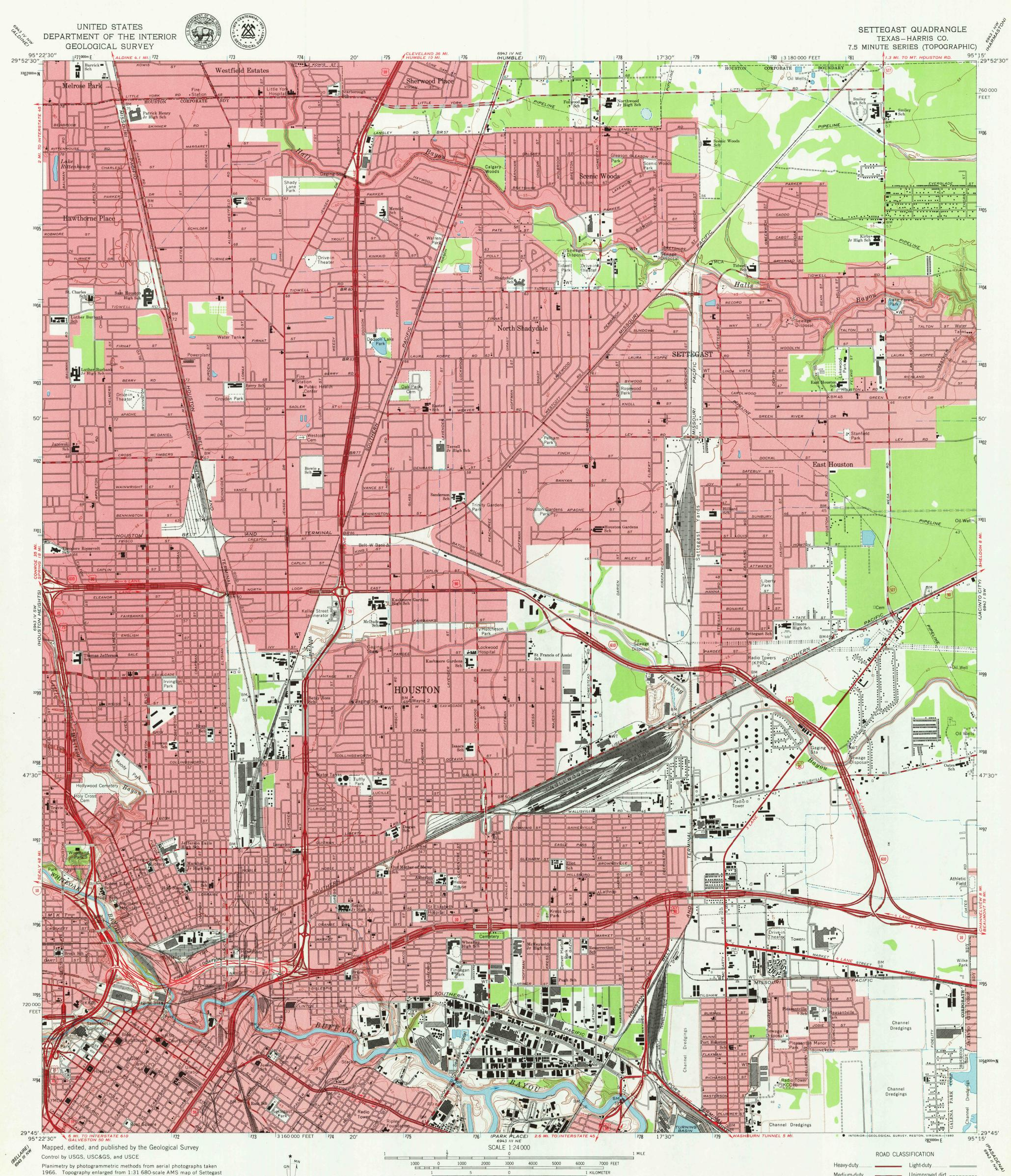
Quadrangle. Original map by planetable surveys 1943. Revised 1967 Polyconic projection. 1927 North American datum 10,000-foot grid based on Texas coordinate system, south central zone 1000-meter Universal Transverse Mercator grid ticks, zone 15, shown in blue
