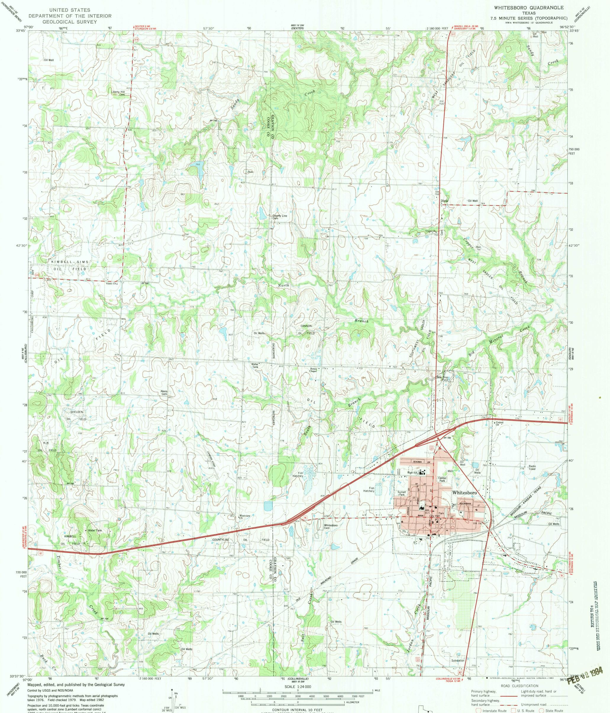
Projection and 10,000-foot grid ticks: Texas coordinate system, north central zone (Lambert conformal conic) 1000-meter Universal Transverse Mercator grid, zone 14 1927 North American Datum To place on the predicted North American Datum 1983 move the projection lines 8 meters south and 27 meters east as shown by dashed corner ticks
