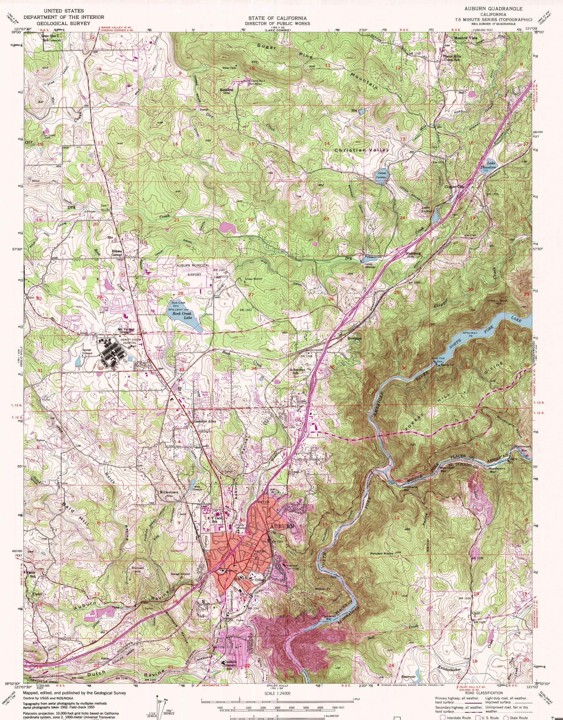
Mercator grid ticks, zone 10, shown in blue. 1927 North American Datum. To place on the predicted North American Datum 1983 move the projection lines 15 meters north and 91 meters east as shown by dashed corner ticks.
