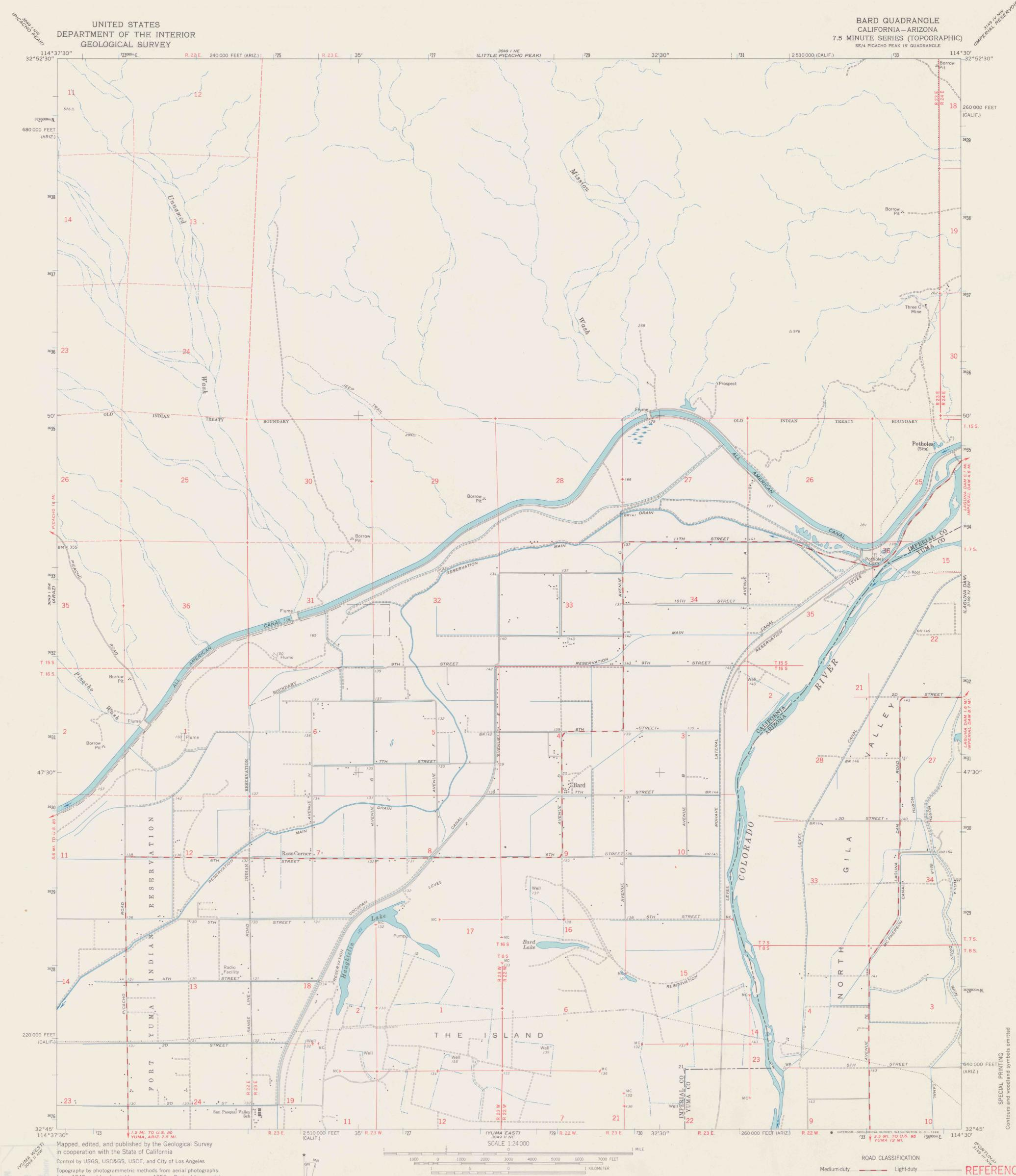
Topography by photogrammetric methods from aerial photographs taken 1948, and by planetable surveys 1952. Revised from aerial photographs taken 1961, and by planetable surveys 1965
