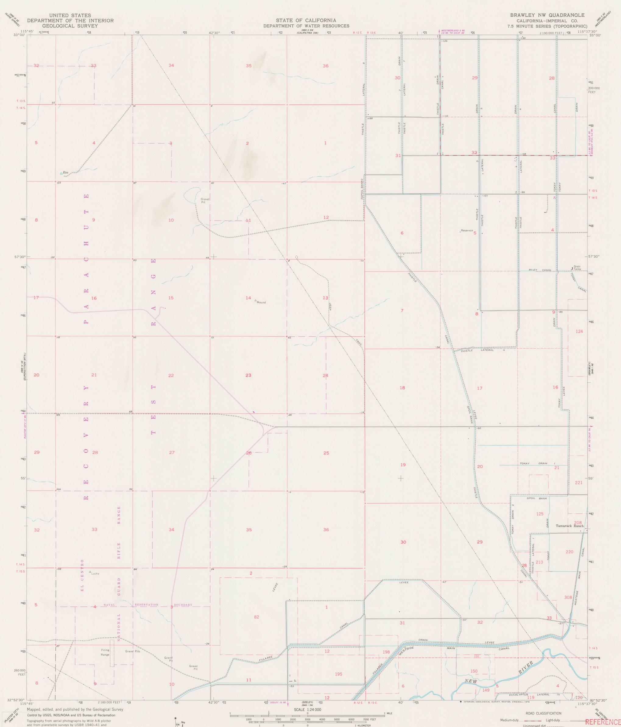
and from planetable surveys by USBR 1940–41 and USGS 1957. Aerial photographs taken 1953 Polyconic projection. 1927 North American datum 10,000-foot grid based on California coordinate system, zone 6 1000-meter Universal Transverse Mercator grid ticks, zone 11, shown in blue To place on the predicted North American Datum 1983 move the projection lines 4 meters south and 76 meters east as shown by dashed corner ticks There may be private inholdings within the boundaries of
