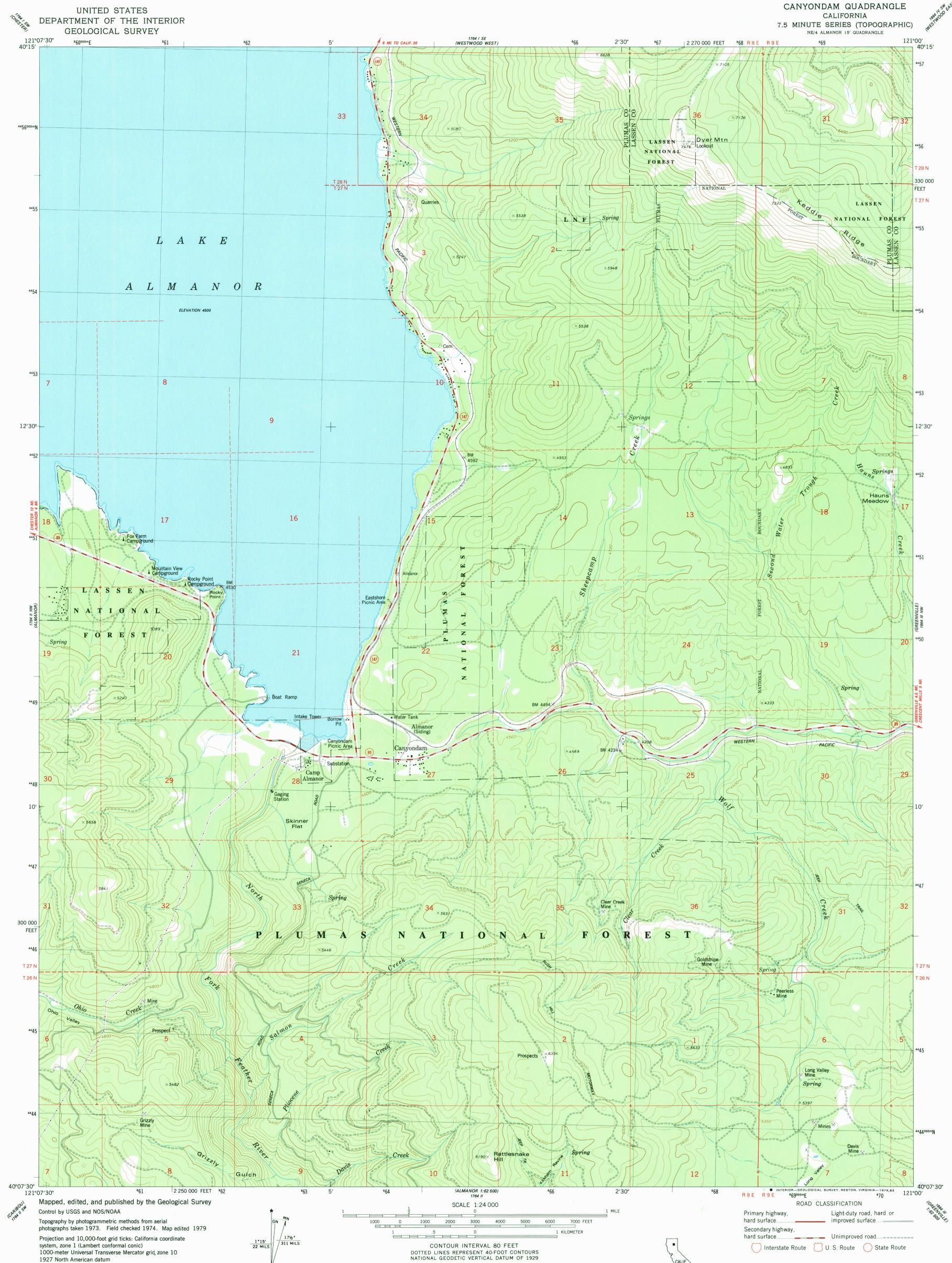
1927 North American datum To place on the predicted North American Datum 1983 move the projection lines 16 meters north and 90 meters east as shown by dashed corner ticks
