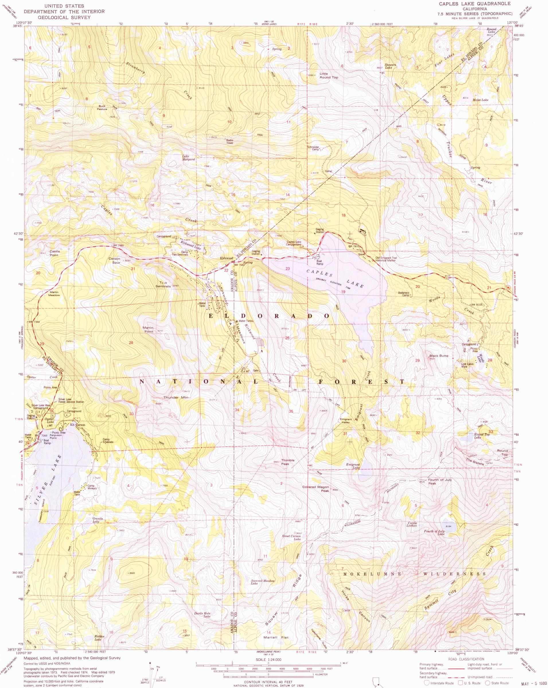
1000-meter Universal Transverse Mercator grid, zone 10 1927 North American Datum To place on the predicted North American Datum 1983 move the projection lines 13 meters north and 88 meters east as shown by dashed corner ticks
