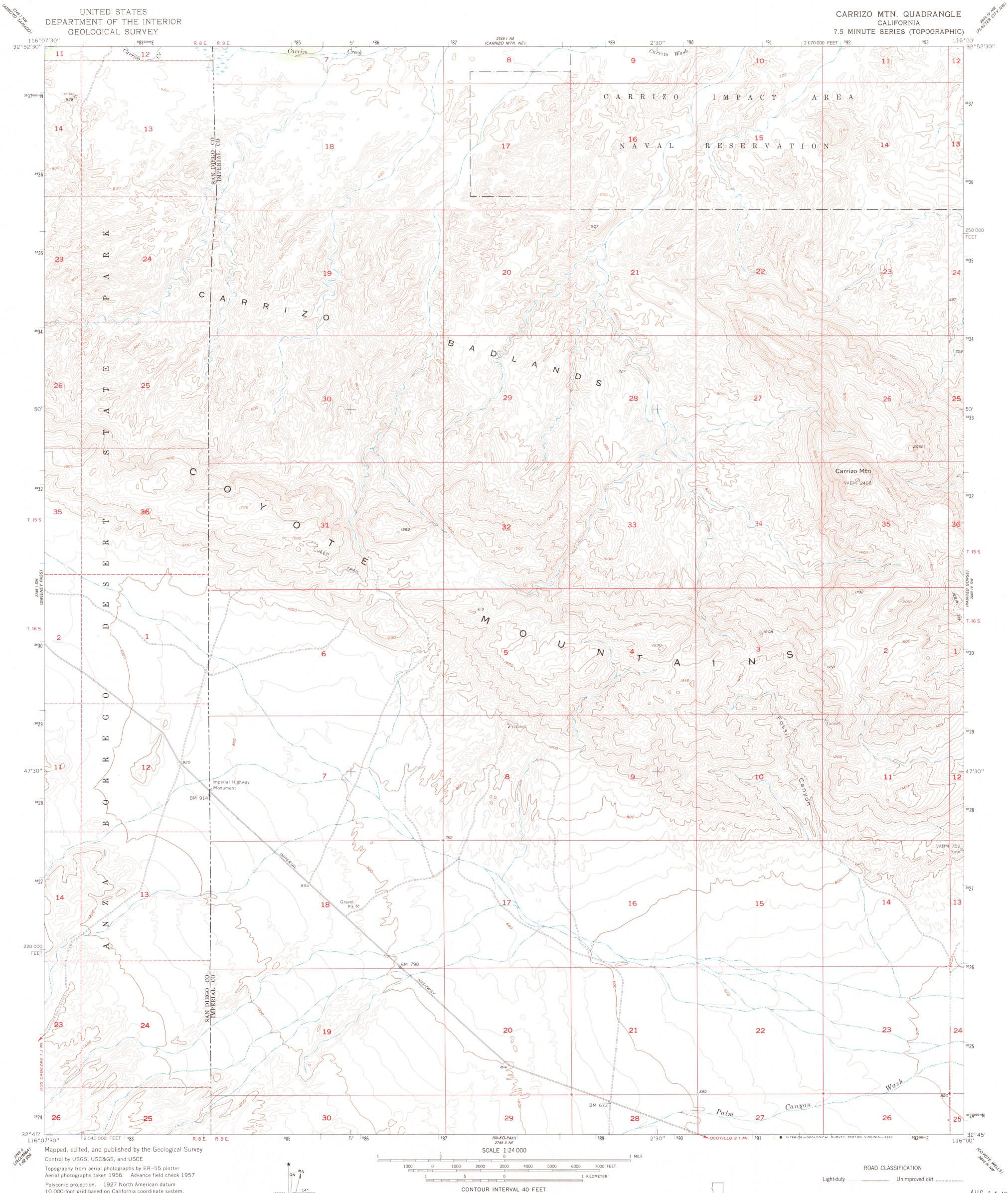
10,000-foot grid based on California coordinate system, zone 6 1000-meter Universal Transverse Mercator grid ticks, zone 11, shown in blue To place on the predicted North American Datum 1983 move the projection lines 4 meters south and 77 meters east as shown by dashed corner ticks There may be private inholdings within the boundaries of the National or State reservations shown on this map
