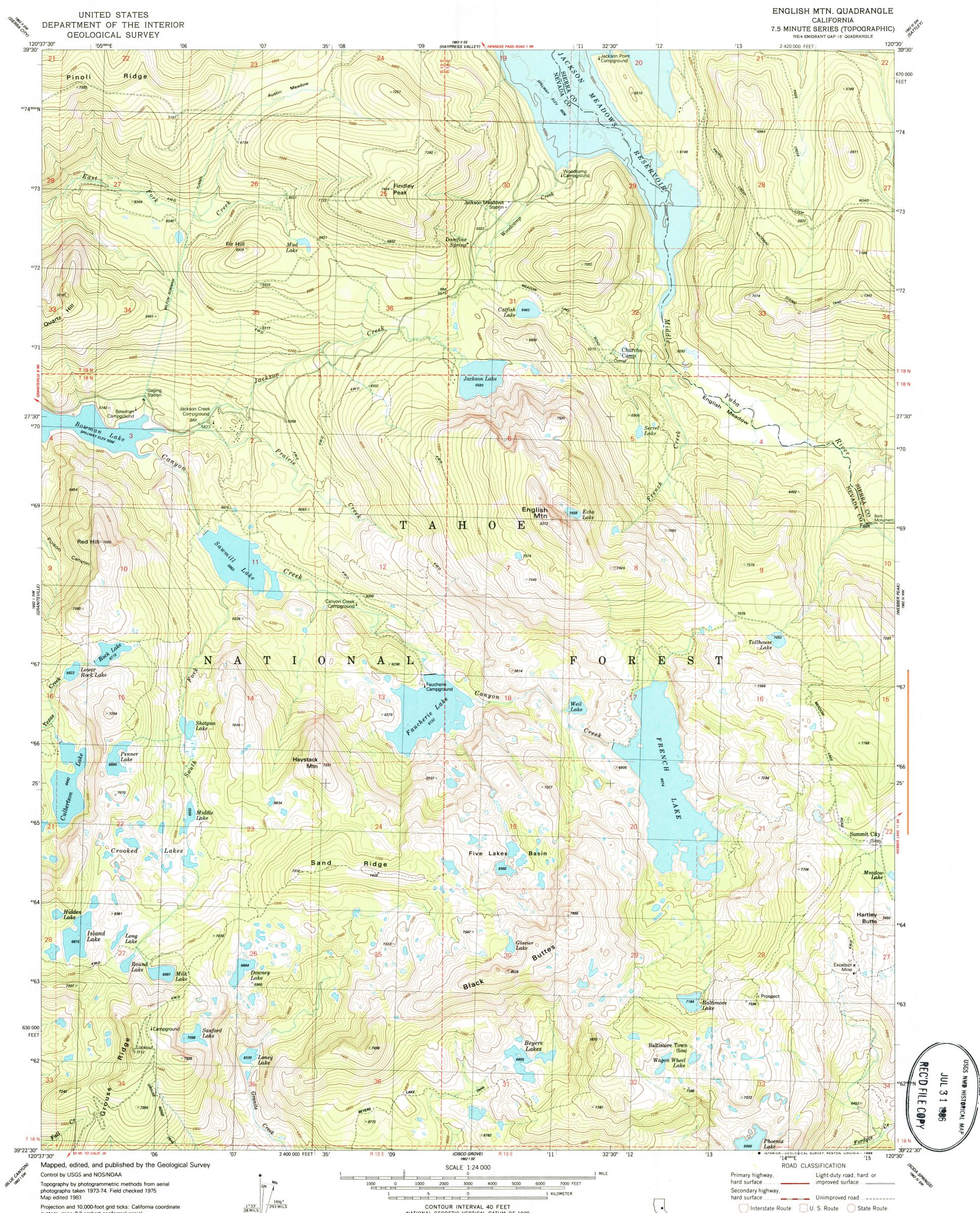
system, zone 2 (Lambert conformal conic) 1000-meter Universal Transverse Mercator grid , zone 10 1927 North American Datum To place on the predicted North American Datum 1983 move the projection lines 15 meters north and 89 meters east as shown by dashed corner ticks
