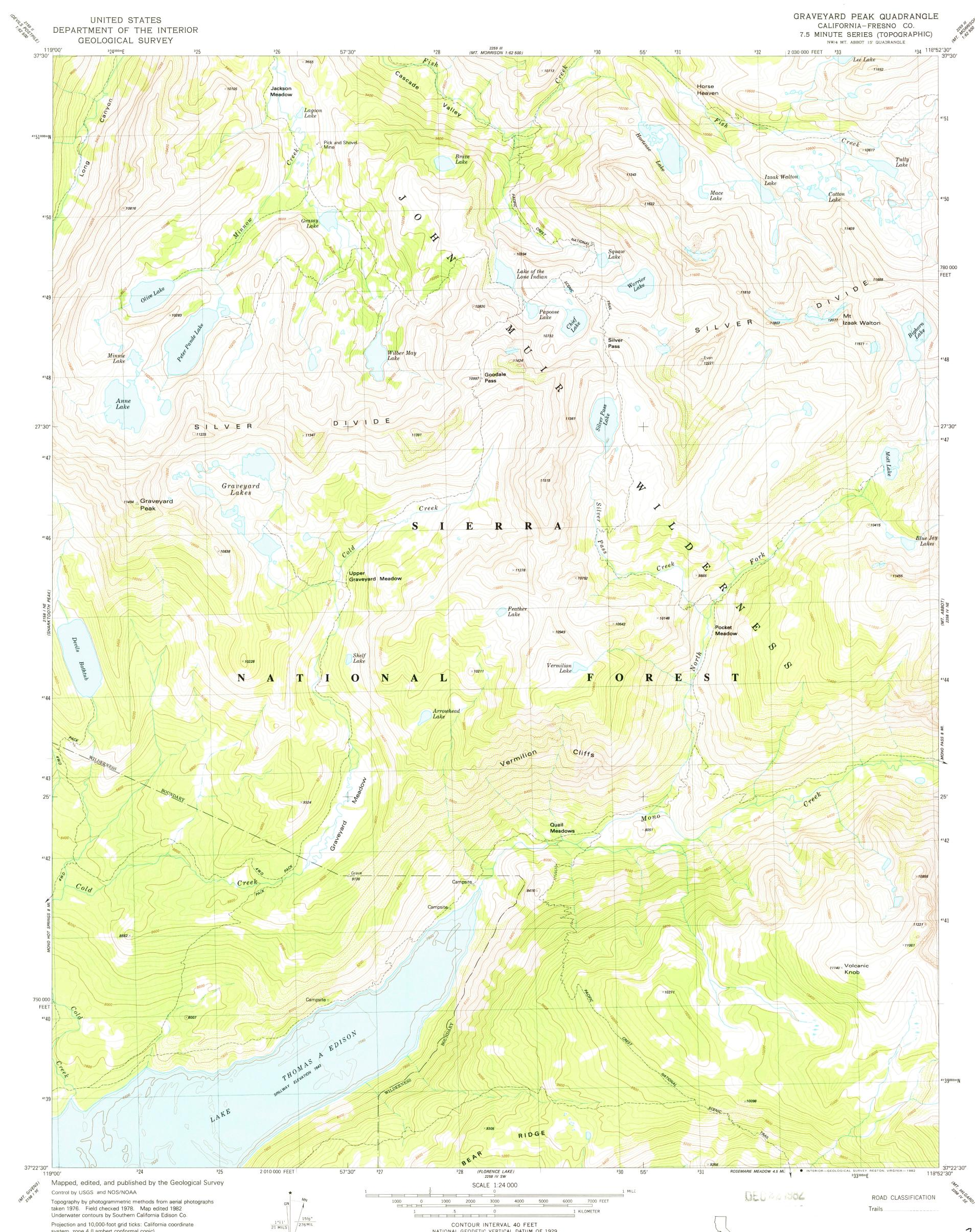
Projection and 10,000-foot grid ticks: California coordinate system, zone 4 (Lambert conformal conic) 1000-meter Universal Transverse Mercator grid, zone 11 1927 North American Datum To place on the predicted North American Datum 1983 move the projection lines 10 meters north and 85 meters east as shown by dashed corner ticks
