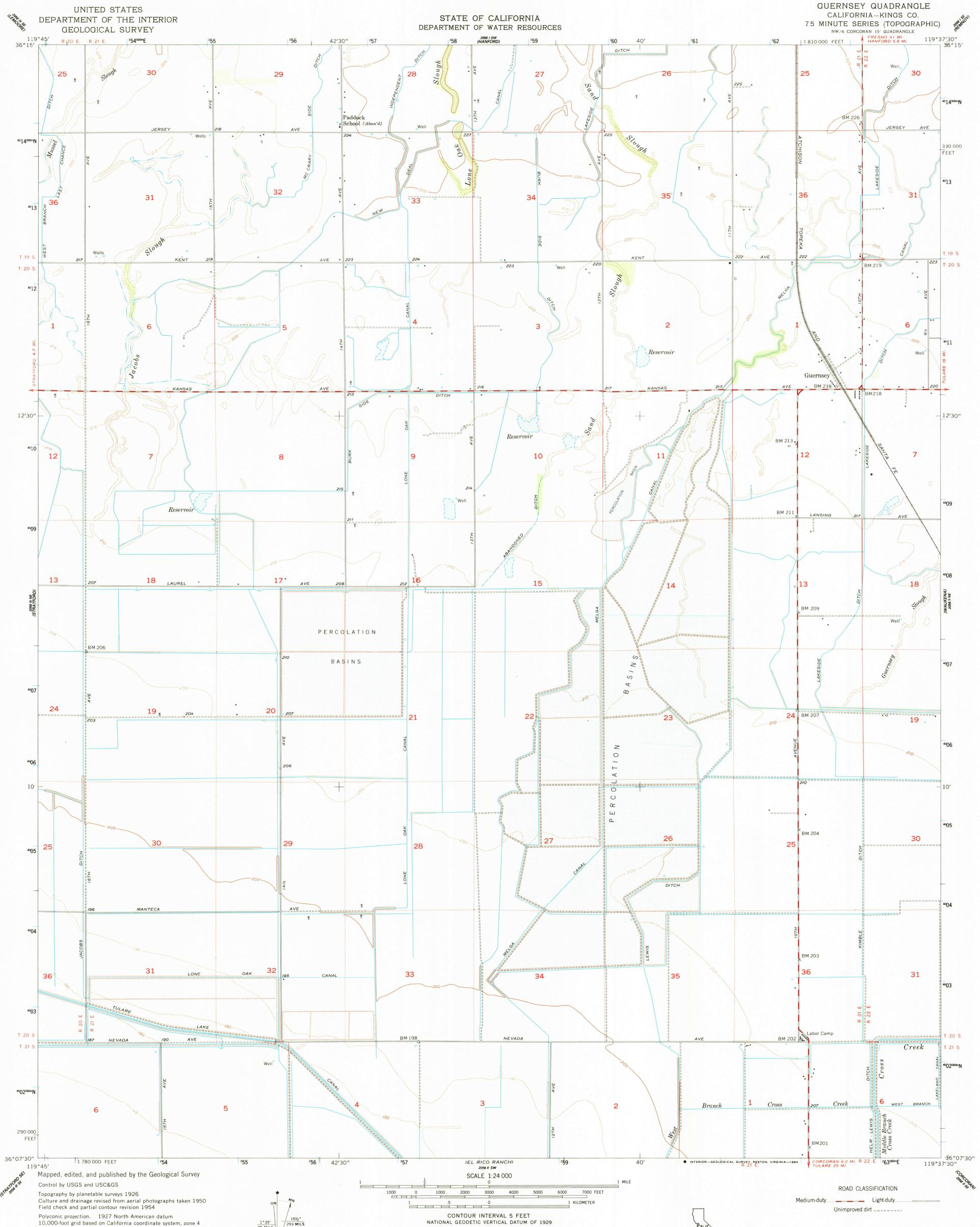
10,000-foot grid based on California coordinate system, zone 4 1000-meter Universal Transverse Mercator grid ticks, zone 10, shown in blue To place on the predicted North American Datum 1983
